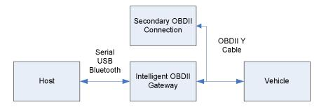
Vehicle status parameters, such as the MIL and DTCs, will be updated from the vehicle once per minute. The host can request these parameters from the OBDII Streamer at any rate desired.
