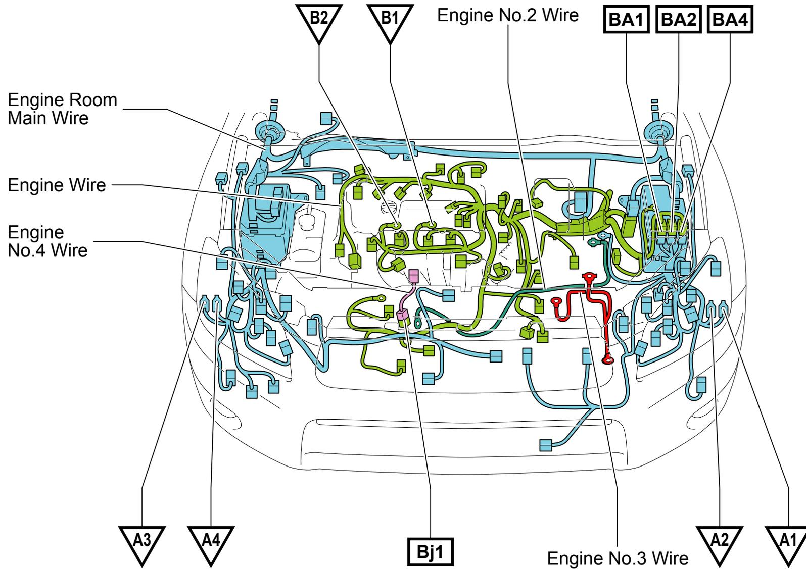
Wire and Wire , Ground Points in Engine Compartment <RHD 3ZR-FAE>
