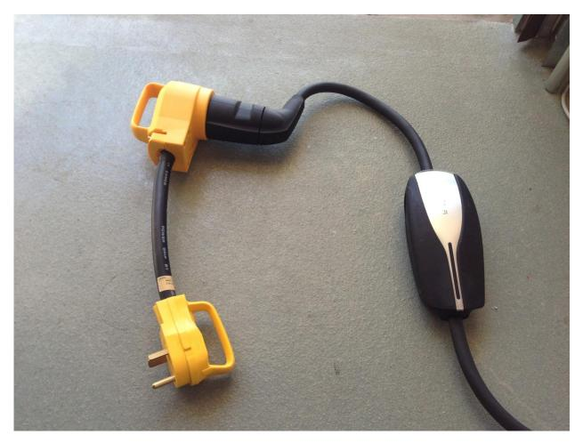
The home made adapter is on the left with the yellow NEMA 14-50 receptacle, wire and yellow adapter plug. The black Tesla NEMA 14-50 adapter and Tesla mobile charger (UMC) are plugged into it.
