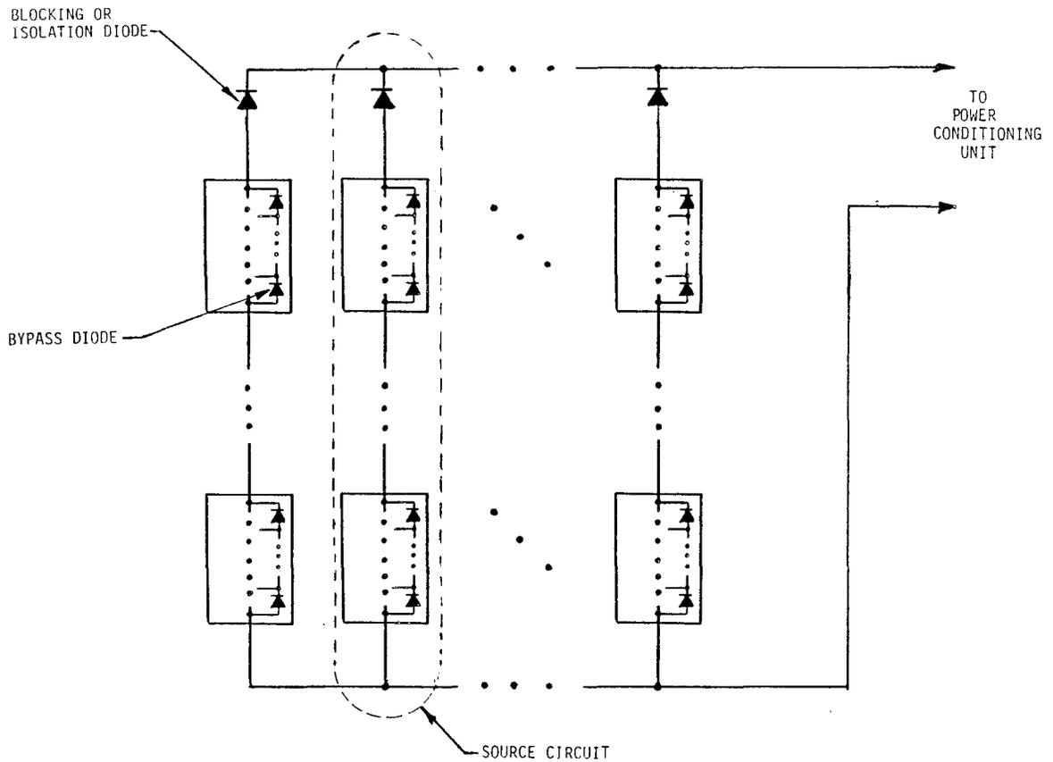
Figure 3-1. Arrangement of Diodes in Photovoltaic Array Circuits
