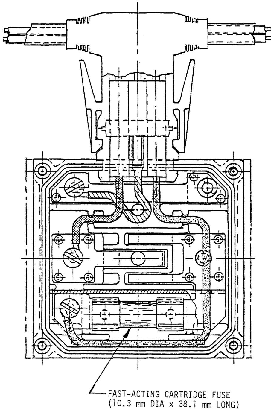
Figure 3-28. The Module-Mounted, Pluggable Diode Enclosure
