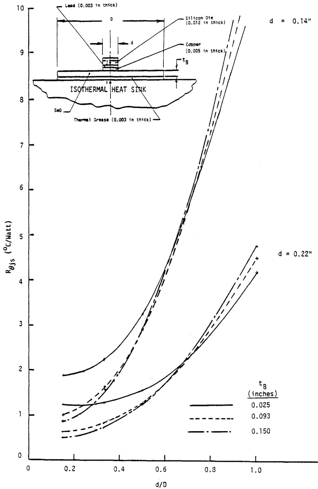
Figure 3-14. Thermal Resistance of the Diode Cell/Beryllia Disk Assembly
