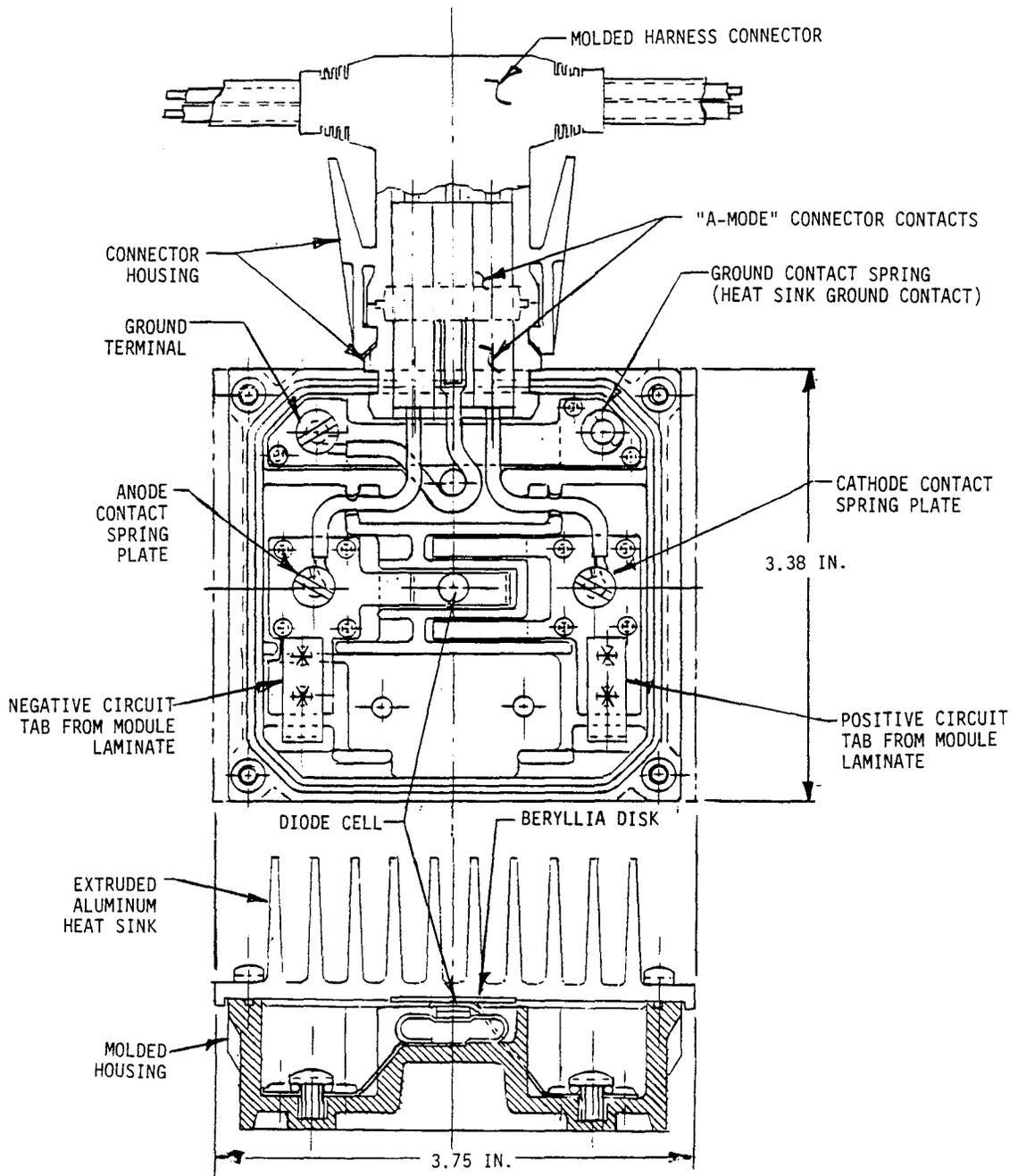
Figure 3-19. Module-Mounted, Pluggable Bypass Diode Enclosure
