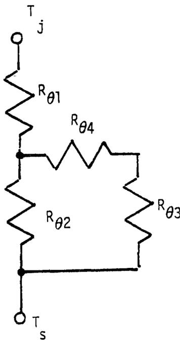
Figure 3-13. Equivalent Circuit Representing the Thermal Resistance Between the Diode Junction and the Isothermal Heat Sink
