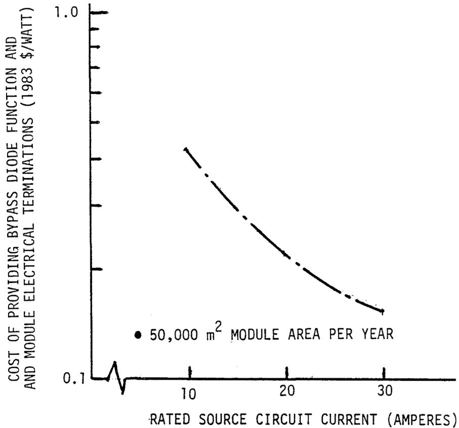
Figure 1-4. Cost of Providing the Bypass Diode Function and Module Electrical Terminations
