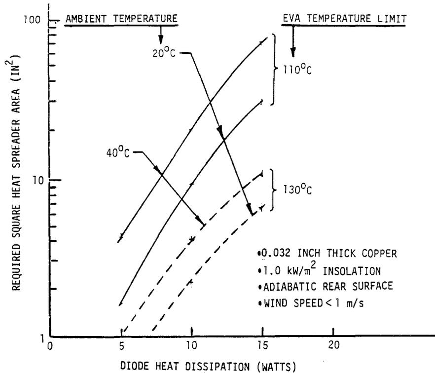
Figure 3-7. Recommended Encapsulated Diode Heat Spreader Plate Size
