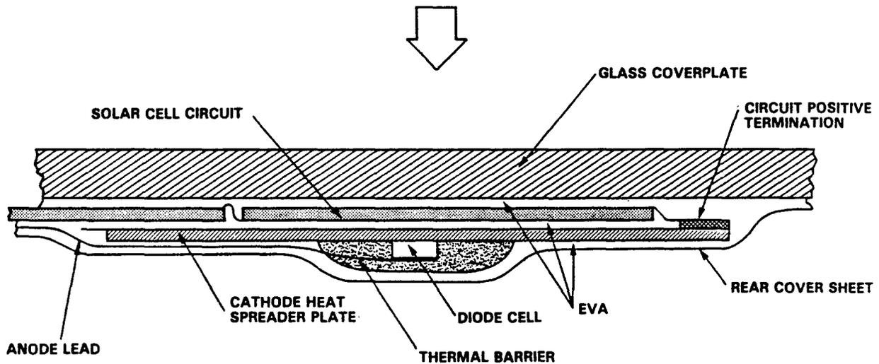
Figure 1-2. Encapsulated Bypass Diode Packaging Approach
