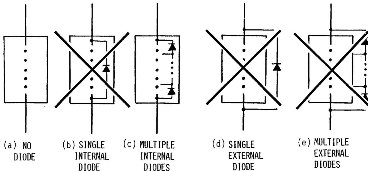
Figure 3-2. The Module Designer's Bypass Diode Options
