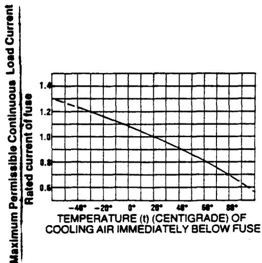
Figure 3-27. Typical Semiconductor Fuse Current Derating Factor
