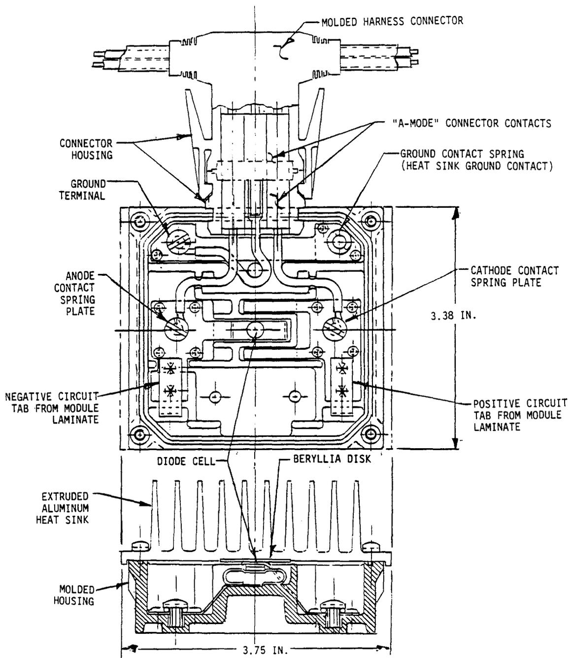
Figure 1-3. Module-Mounted, Pluggable Bypass Diode Enclosure
