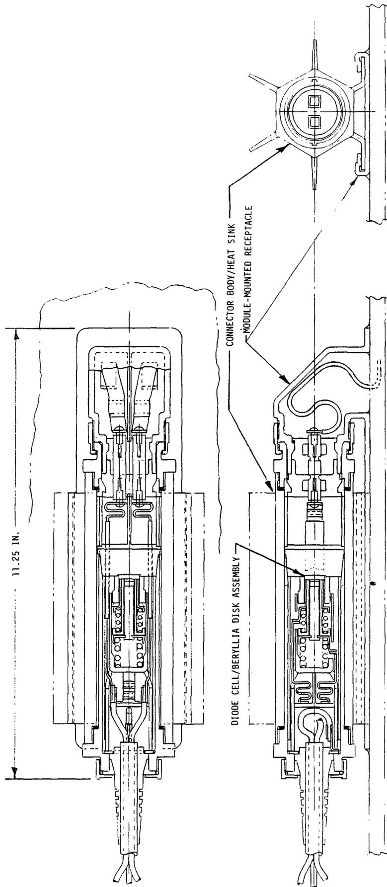
Figure 3-22. Harness-Mounted, Connector-Integrated Bypass Diode Package
