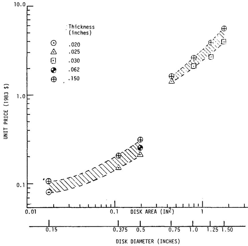
Figure 3-17. Price of BeO Insulating Disks for a Quantity of 50,000 Units
