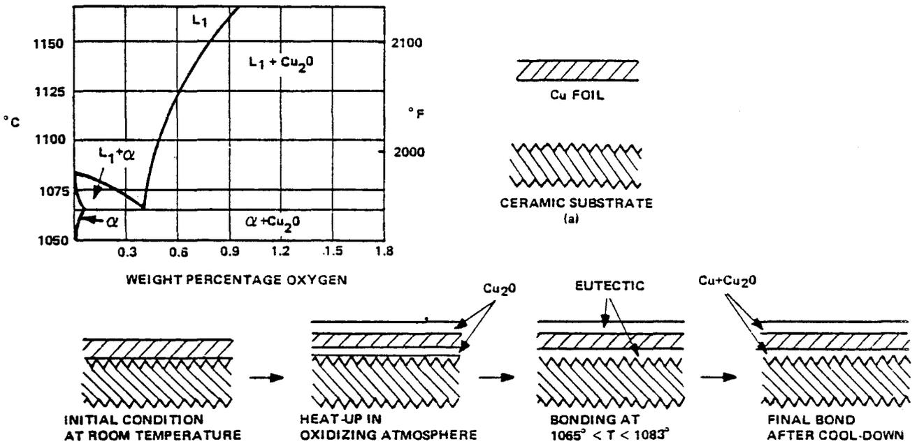
Figure 3-11. Direct-Bonded Copper
