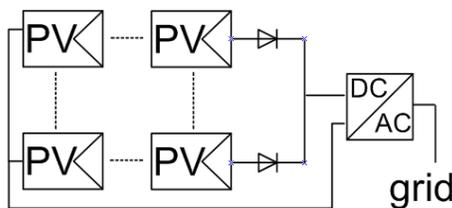
Fig. 2. Centralized Inverters
