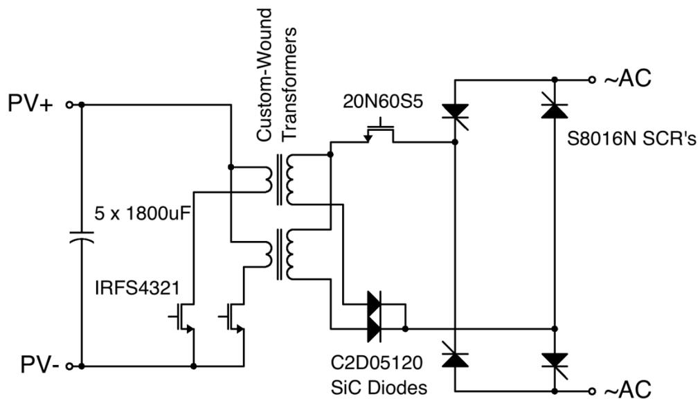
Fig. 11. Enphase micro-inverter fly-back topology
