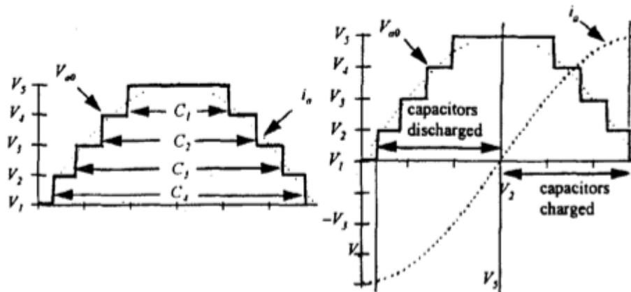
Fig. 8. Operation waveform of the 5-step diode-clamped inverter
