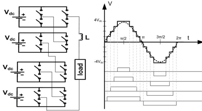
Fig. 6. Cascade H-bridge multilevel inverter and operation
