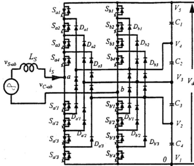
Fig. 7. 5-step diode-clamped inverter topology
