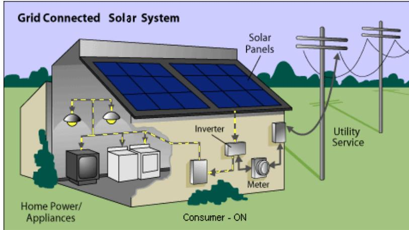
Fig. 1. Grid connected solar system
