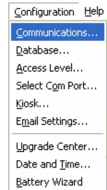
**DATABASE:** Allows changing the 15-minute default value in the *Database* window. The user can specify how often the software averages the M4/M5-Plus data and writes these values to the database. Clicking the *Manual Write DB averages* button forces a one time immediate averaging and writing of the M4/M5-Plus data to the database.
