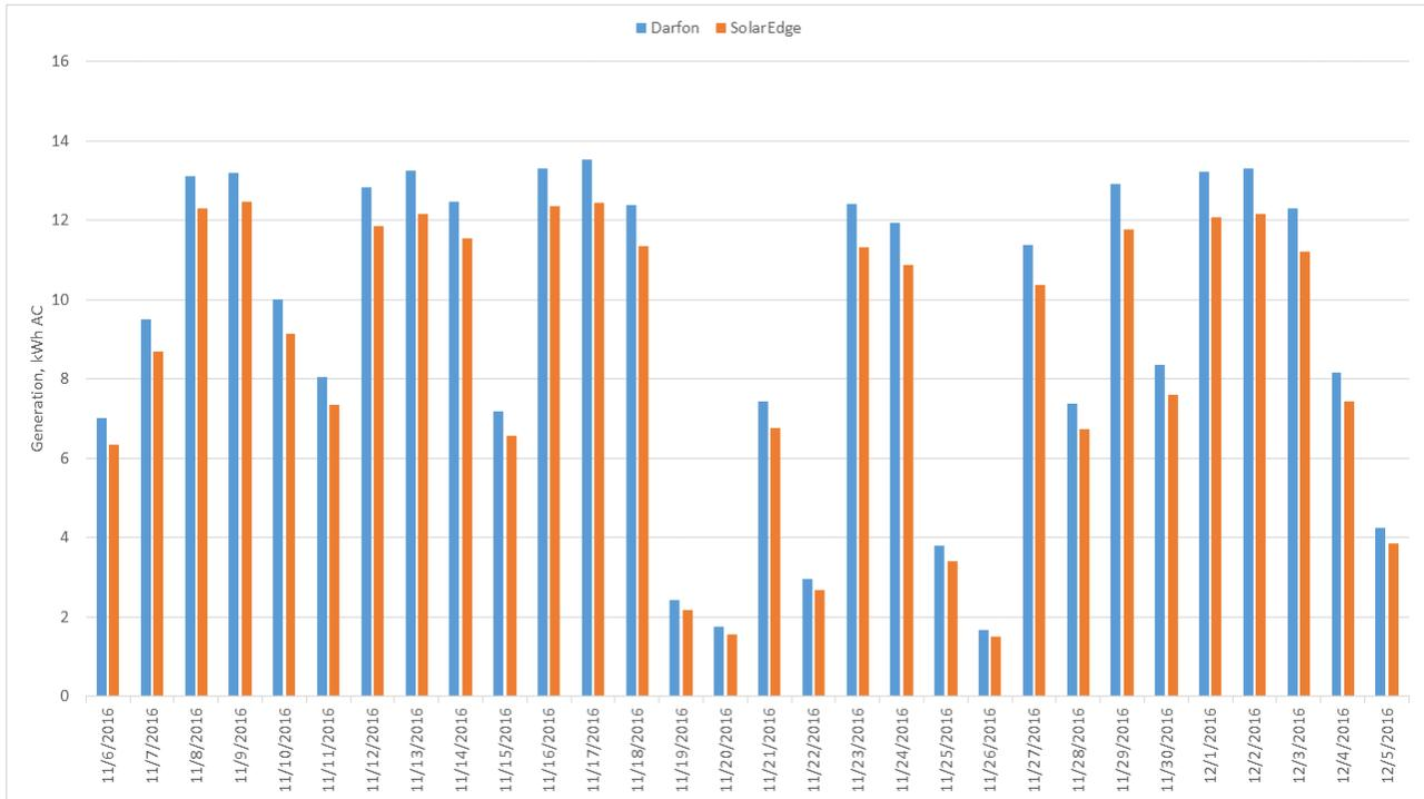
Figure 2. Daily energy generated from Darfon G320 MI vs SolarEdge 3kW SI
