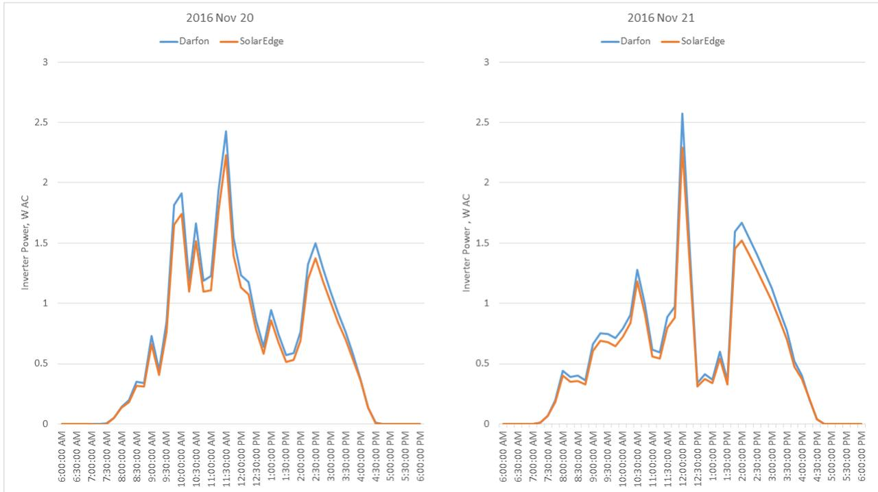
Figure 1. Instantaneous power of Darfon G320 MI vs SolarEdge 3kW SI
