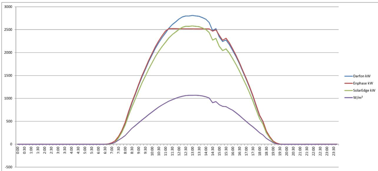
Figure 3. Power output of Darfon G320 vs Enphase M250 vs SolarEdge 3kW.
