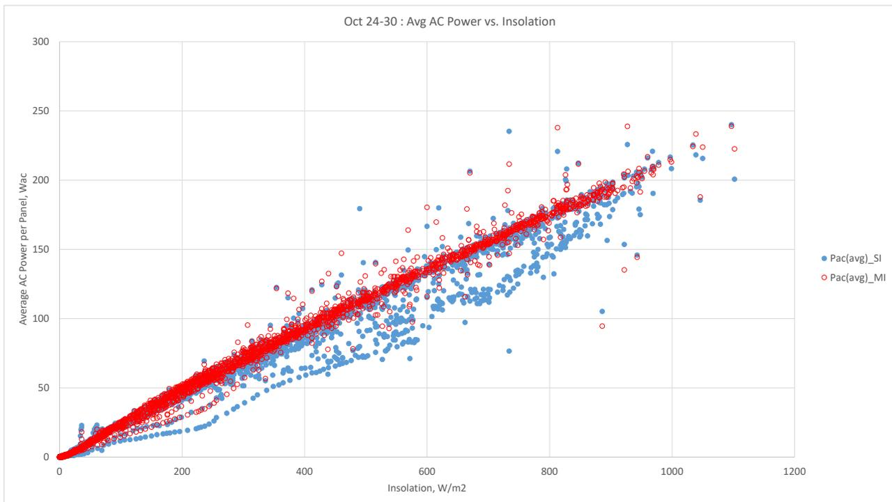
Figure 7. Average AC Power vs Insolation of Darfon MI vs Schneider SI
