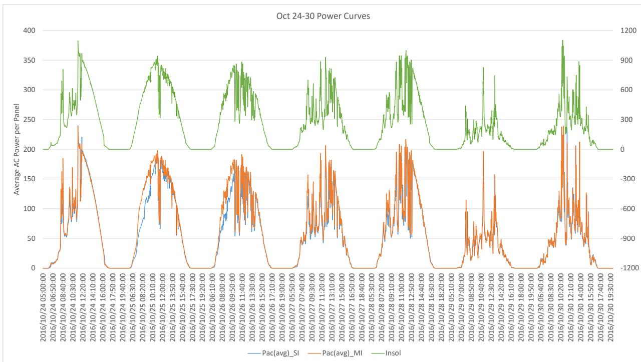
Figure 5. Outdoor data of Darfon G320 micro inverter vs Schneider string inverter
