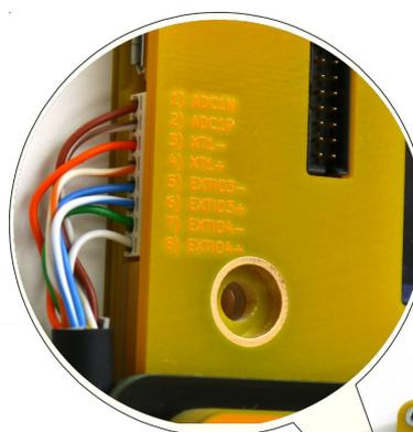
Use a CAT5 or CAT6 Ethernet cable with the 8 pin connector. All you need to do is strip 4 to 5 mm from the end of the wire and insert in the connector until the stop is reached. To remove the wires insert a needle in the corresponding rectangular hole above the wire as seen in the third drawing below. Use the 2 (SBMS40) or 3 (SBMS120) provided cable ties to secure the cable to the SBMS case.
