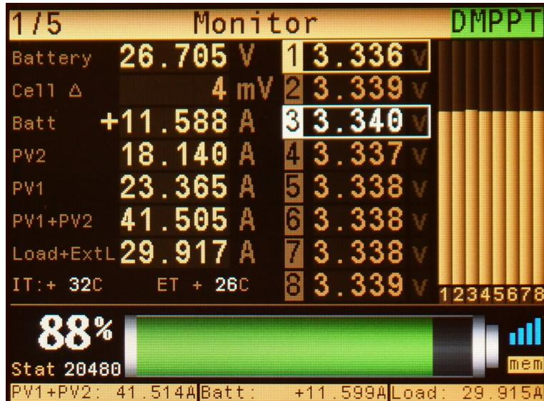
By pressing the OK button while in this menu you will be presented with a small submenu allowing you to change the display from current measured with 1mA resolution to power measured with a 0.1W resolution and also allowing you to change the temperature units from Celsius to Fahrenheit
