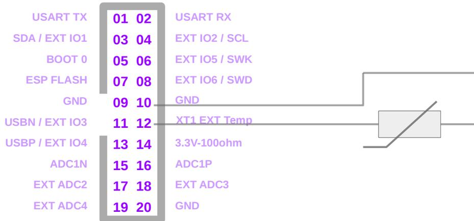
The SBMS is calibrated for a particular 10kOhm thermistor made by Murata NCP21XV103J03RA (this same thermistor type is used internally to measure the power board temperature).
