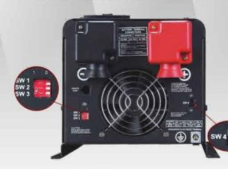
On the DC end of inverter, there are 4 DIP switches which enable users to customize the performance of the device.
