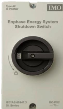
EP200G-NA-02-RSD is the Enphase Energy System Shutdown switch which also provide Rapid shutdown capability for System Controller 2 as required by NEC standard. This component is certified by UL1741 PVRSE requirement. The component also contains necessary labels which are required as per the NEC to identify the Rapid Shut down switch.
