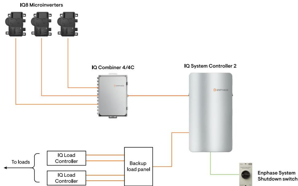
The system consists of IQ8 Series Microinverters, IQ System Controller 2, IQ Combiner 4C, 2x IQ Load Controllers and other accessories as needed.
