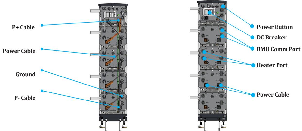
Figure 5.39 Battery Pack Cabling
