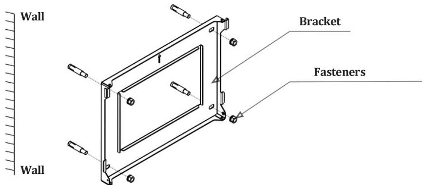
Figure 5.17 Fixing the bracket to the wall
