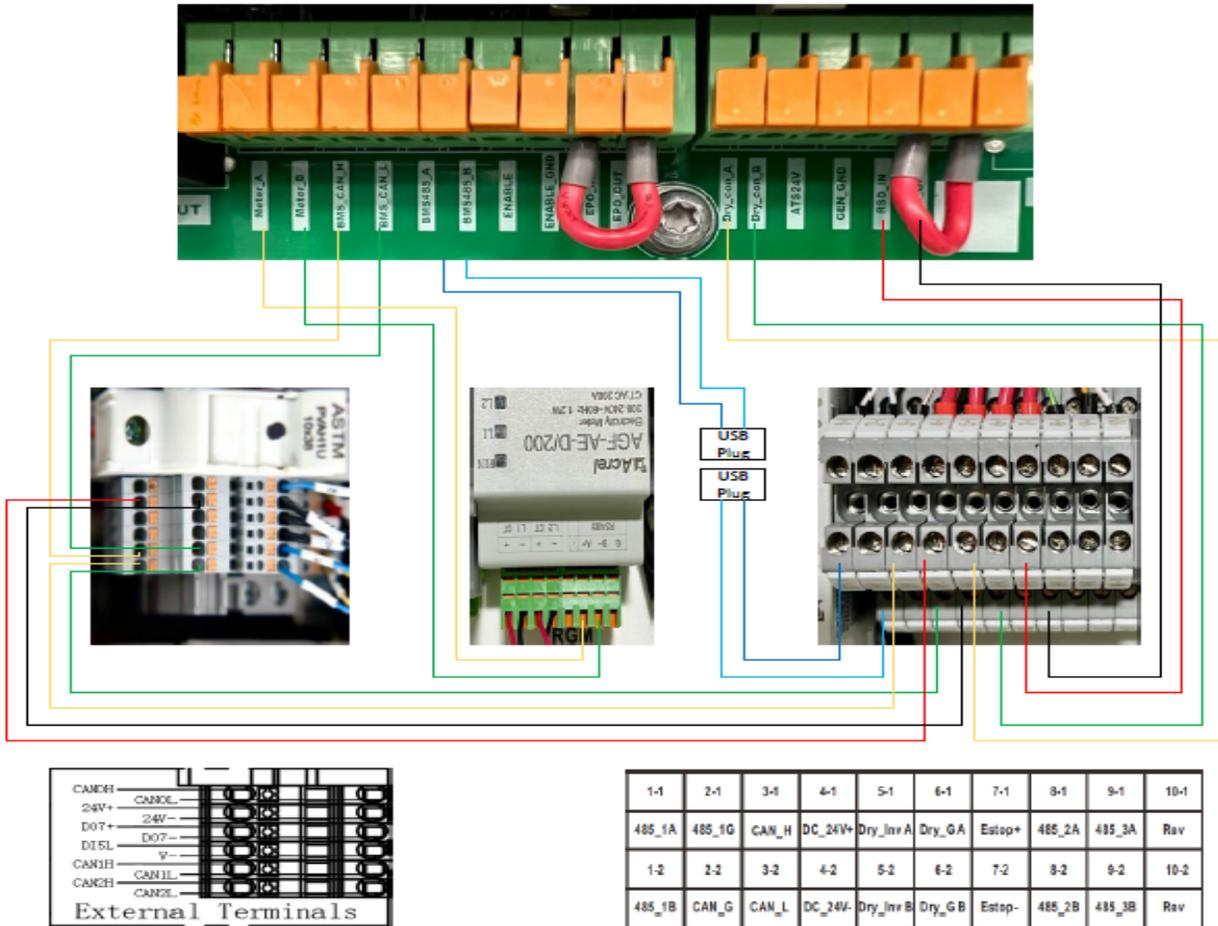
Figure 5.7 SEP Low Voltage and Communication Wiring
