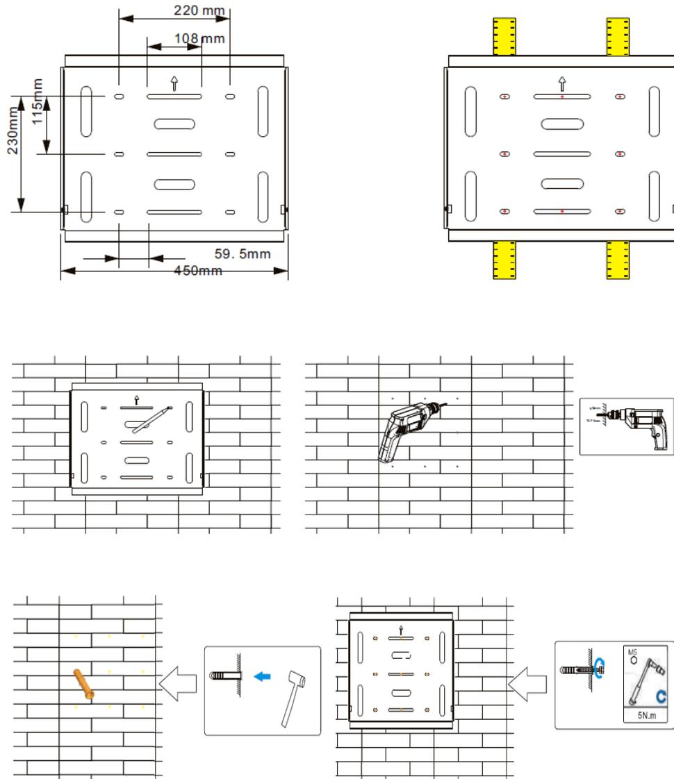
Figure 5.4 Install SEP Mounting Bracket
