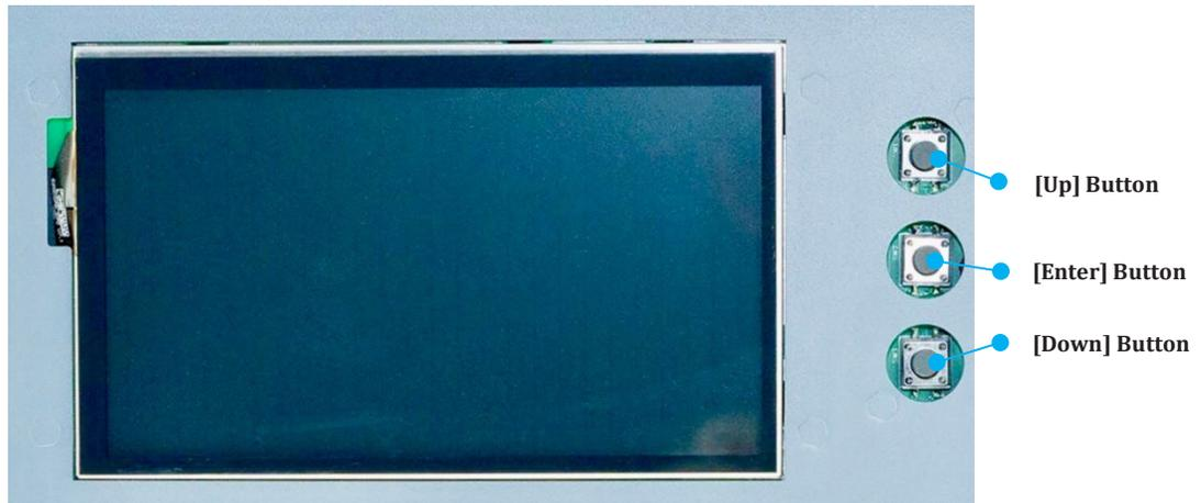
Figure 6.1 SEP HMI LCD Display and Control
