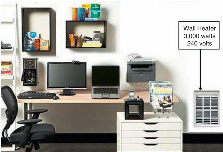
**Figure 9.9** Office heater loads must be based on the total current draw of all the heaters.
