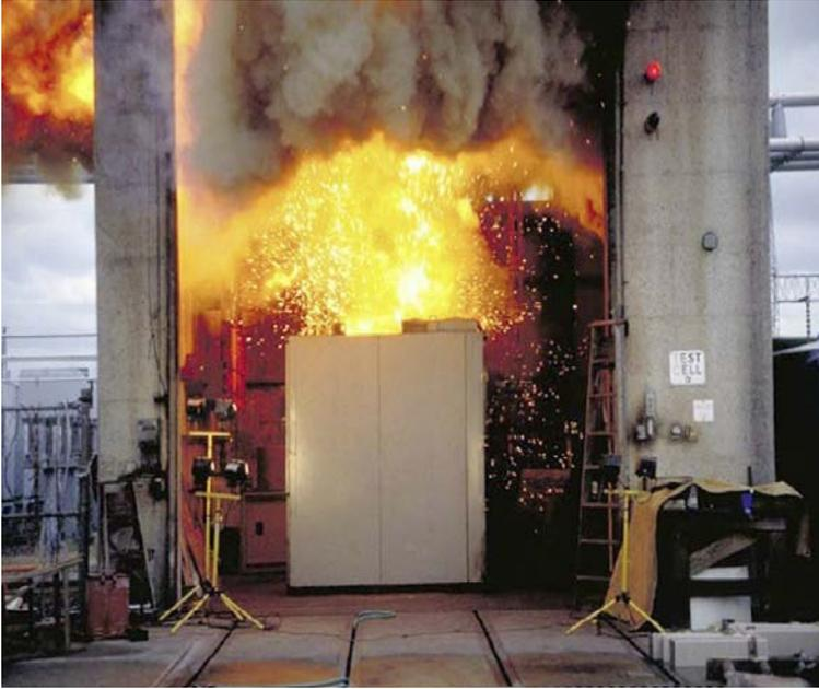
**Figure 7.1** An arc blast causes damage from fire, concussion waves, heat, and liquefied metal.
