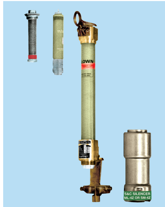
Exhibit 490.2 Components of the indoor solid-material (SM) power fuseholder (boric-acid arc-extinguishing type) with a 14.4 kV, 400E-ampere maximum, 40,000-ampere rms asymmetrical interrupting rating. Shown here are the spring and cable assembly, refill unit, holder, and snuffler. (Courtesy of S&C Electric Co.)
