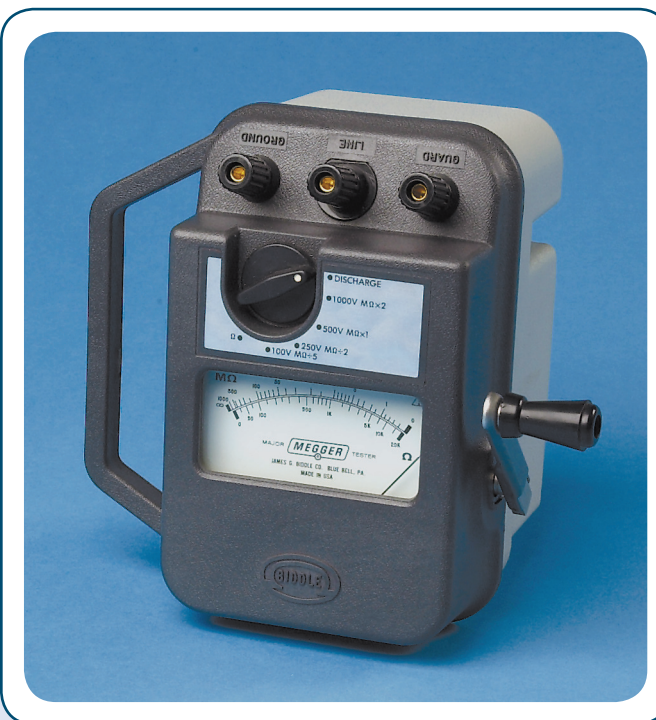
EXHIBIT 110.1 A manual multivoltage, multirange insulation tester.
