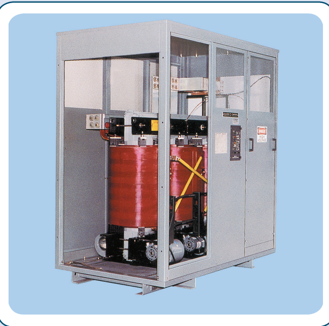
EXHIBIT 450.12 A dry-type transformer with a core and coil design rated at 1000 kVA, 13,800 volts to 480 volts, 3-phase, 60 Hz. Note cooling fans beneath each winding. (Courtesy of Schneider Electric)
