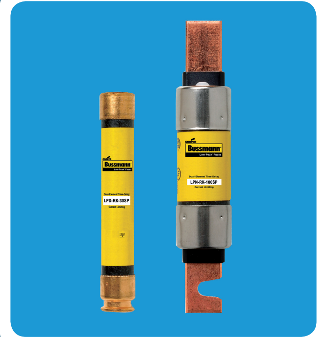
EXHIBIT 240.1 Class R current-limiting fuses with rejection feature to prohibit the installation of non-current-limiting fuses. (Courtesy of Cooper Bussmann, a division of Cooper Industries, PLC)
