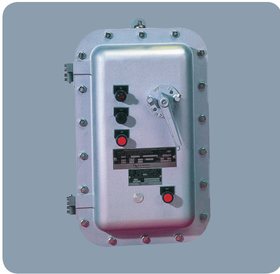
EXHIBIT 501.16 A magnetic motor starter for use in a Class I, Group D location. Note the number of securing bolts and the width of the flange. (Courtesy of O-Z/Gedney, a division of EGS Electrical Group)
