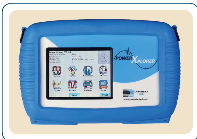
EXHIBIT 310.6 A portable tool for such tasks as diagnostic power analysis, including harmonic distortion. This is one example of a more advanced solution to 310.15(B)(5)(c), where accurate measurement and thorough circuit analysis is desirable. (Courtesy of Dranetz-BMI)
