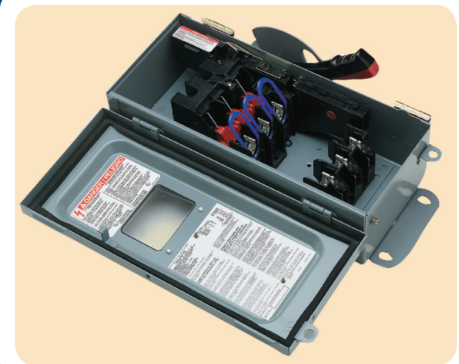
EXHIBIT 430.19 Heavy-duty safety switches, UL-listed for use on systems up to 200,000 amperes fault current rms symmetrical with Class J or Class R fuses installed. (Courtesy of Schneider Electric)
