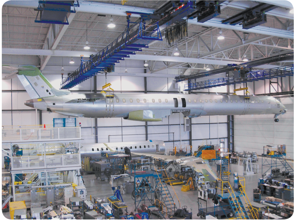
EXHIBIT 610.1 New CRJ1000 NextGen aircraft fuselage being hoisted for joining at Bombardier Aerospace's Mirabel Manufacturing Plant. (Courtesy of Bombardier Aerospace)
