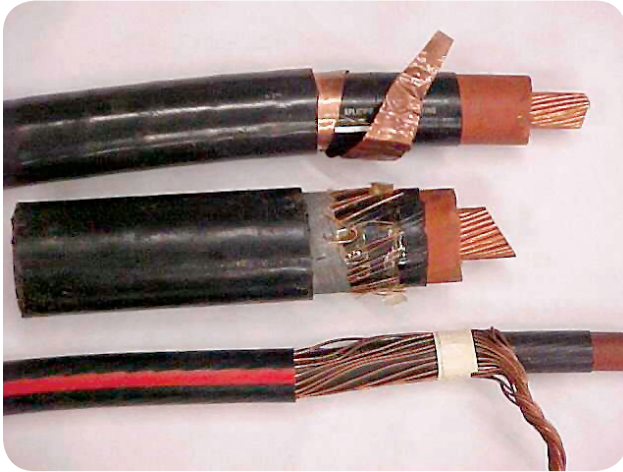
EXHIBIT 250.61 Three examples of single-conductor shielded cable each having a different type of shielding. (Courtesy of Chuck Mello)
