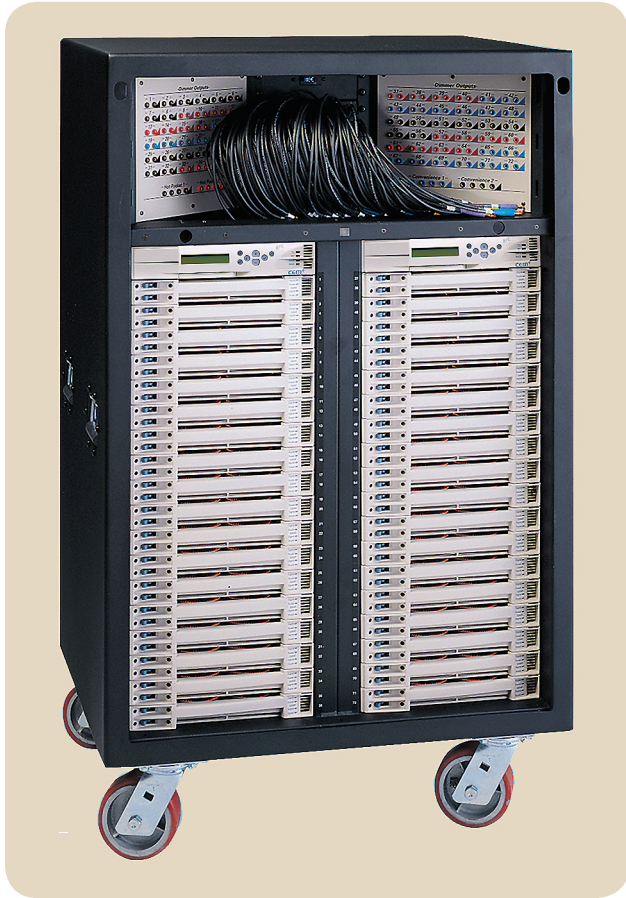
EXHIBIT 520.11 A large, portable SCR dimmer switchboard (rolling rack). (Courtesy of Electronic Theatre Controls, Inc.)
