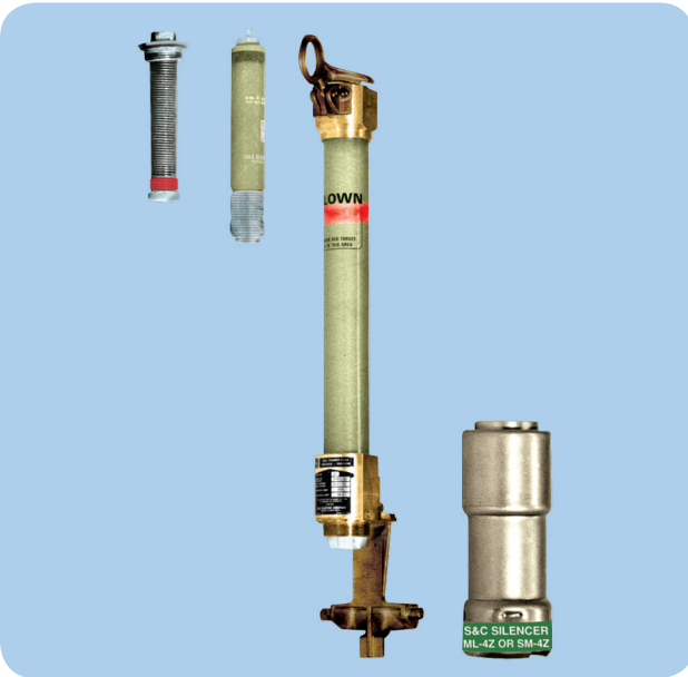
EXHIBIT 490.2 Components of the indoor solid-material (SM) power fuseholder (boric-acid arc-extinguishing type) with a 14.4 kV, 400E-ampere maximum, 40,000-ampere rms asymmetrical interrupting rating. Shown here are the spring and cable assembly, refill unit, holder, and snuffler. (Courtesy of S&C Electric Co.)
