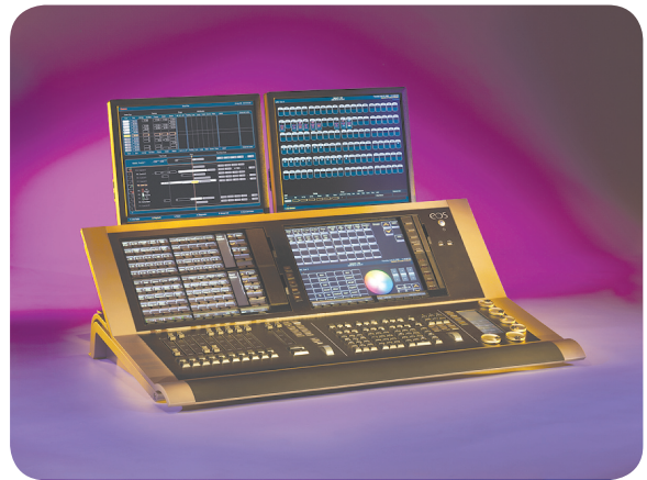
EXHIBIT 520.4 An electronic computer lighting control console for remotely controlling solid-state-type dimmers. (Courtesy of Electronic Theatre Controls, Inc.)
