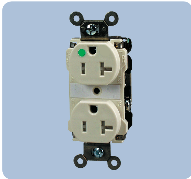
EXHIBIT 517.2 A tamper-resistant hospital-grade receptacle, identified by a green dot on its face, that fulfills the requirements of 517.18(B) and (C). (Courtesy of Legrand/Pass & Seymour®)
