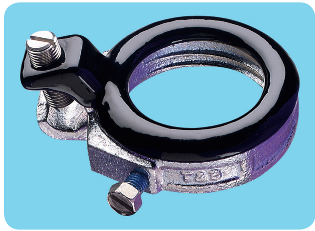
EXHIBIT 250.38 A threaded grounding bushing with set screws used to ensure electrical and mechanical connection and a terminal for connection of a grounding conductor or bonding jumper. (Courtesy of Thomas & Betts Corp.)
