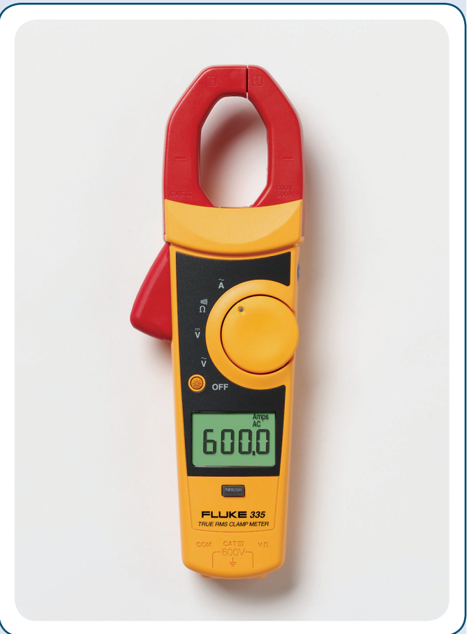
EXHIBIT 310.5 A clamp-on ammeter that uses true rms measurements. This is an example of one solution to 310.15(B)(4)(c), where accurate measurement of neutral current becomes necessary. (Courtesy of Fluke Corp.)
