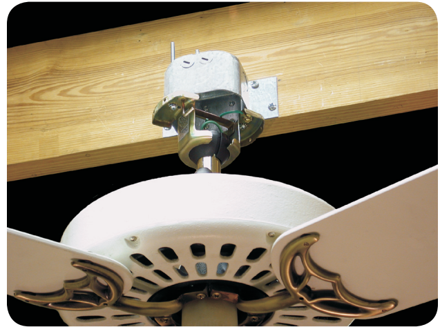
EXHIBIT 422.2 Supporting a ceiling-suspended (paddle) fan (35 lb or less) with a box identified for such use, per 422.18. (Courtesy of Hubbell RACO)
