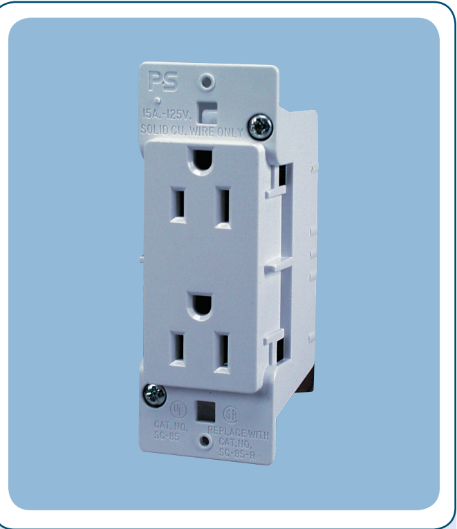
EXHIBIT 300.14 A self-contained device (SCD) receptacle, one example of a boxless device permitted by 300.15(E). (Courtesy of Legrand/Pass & Seymour®)
