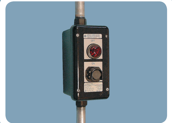
EXHIBIT 502.3 A dust-ignitionproof pushbutton control station suitable for use in Class II, Group E, F, and G locations. (Courtesy of Appleton Electric Co., EGS Electrical Group)
