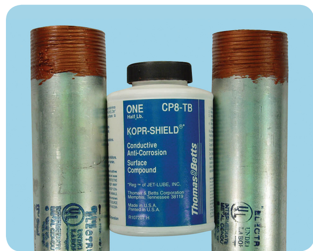
EXHIBIT 300.11 KOPR-Shield® (a registered trademark of Jet Lube), a conductive anti-corrosion surface compound suitable for application on field-cut conduit threads where protection from corrosion is necessary according to 300.6(A). (Courtesy of Thomas & Betts Corp.)
