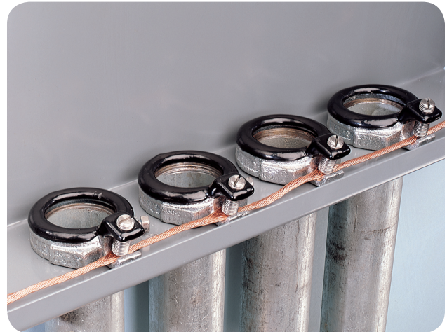
EXHIBIT 250.37 Grounding bushings used to connect a copper bonding or grounding wire to conduits. (Courtesy of Thomas & Betts Corp.)
