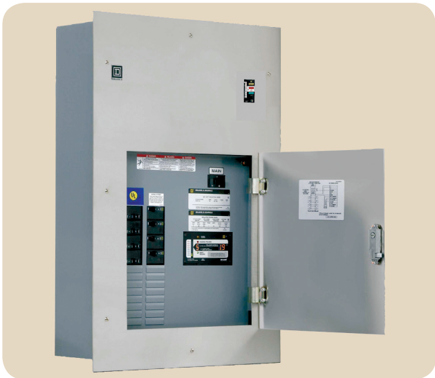
EXHIBIT 517.7 An example of a hospital isolated power system panel with built-in isolation transformer, line isolation monitor, load center, and grounded busbar. (Courtesy of Schneider Electric)
