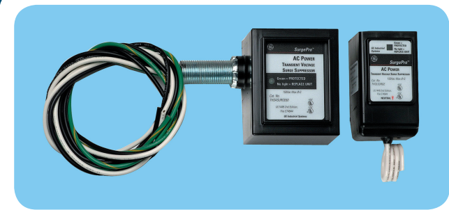
EXHIBIT 285.1 Two SPDs suitable for service-entrance installation, one for direct connection to panelboard busbars and one for mounting in a cabinet or enclosure knockout. (Courtesy of General Electric)
