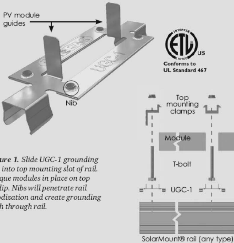
Figure 1. Slide UGC-1 grounding clip into top mounting slot of rail. Torque modules in place on top of clip. Nibs will penetrate rail anodization and create grounding path through rail.
