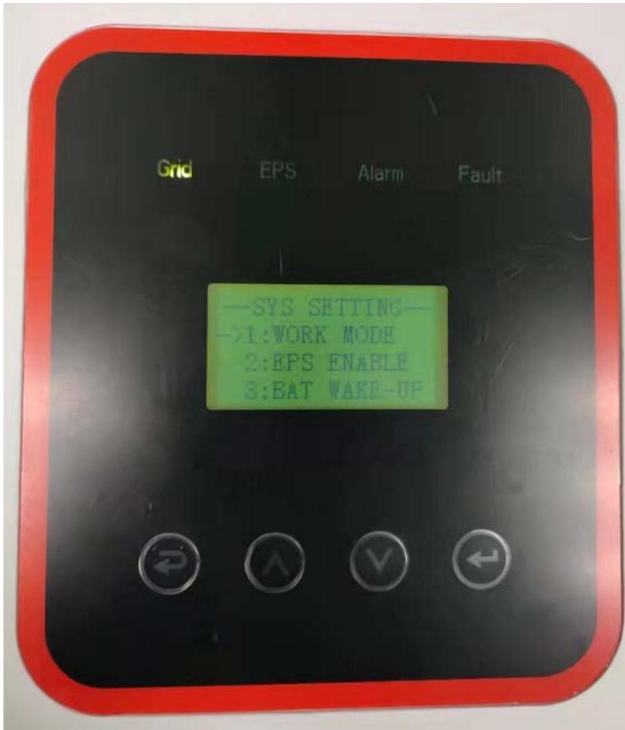
3.1.1 After entering WORK MODE, SELF CONSUME (spontaneous use), PEAK SHIFI (peak shaving and valley filling is grid-connected discharge mode) and BAT PRIORITY will be displayed. In PEAK SHIFI mode, there will be WORK TIME options, namely Time 1, Time 2 and Time 3.
