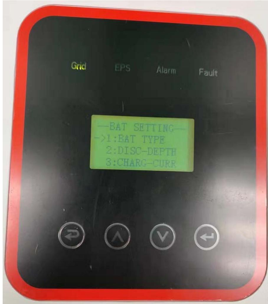
3.2.1 Enter the BAT SETTING interface, click BAT TYPE to select the corresponding battery.
