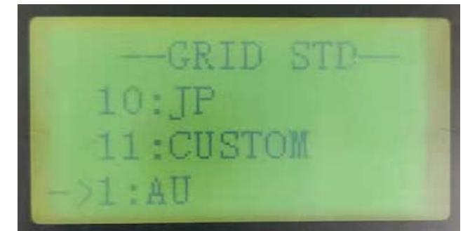
3.4 Click GRID SET to enter the GRID SET interface and select the corresponding voltage.
