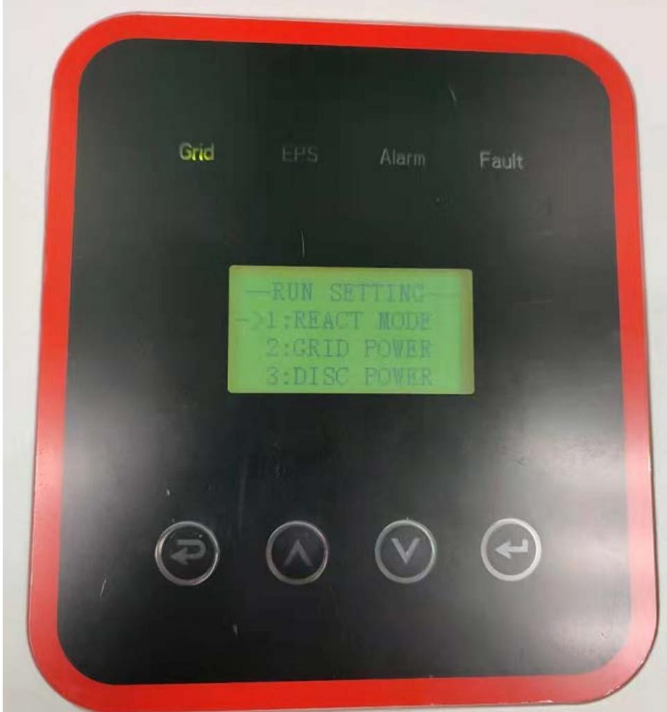
3.5.1 Click REACT MODE to enter the REACT MODE interface. There are a total of 4 options, namely POWER FACTOR, REACT POWER, QU WAVE and QP WAVE.
