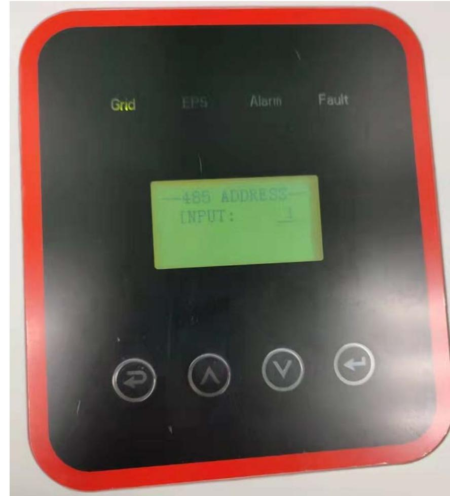
3.7 Click BAUD RATE to enter the SELECT interface, select the baud rate 9600.
