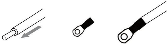
**Step2.** Cross the battery cable through the battery port. Connect battery cable to battery terminal
