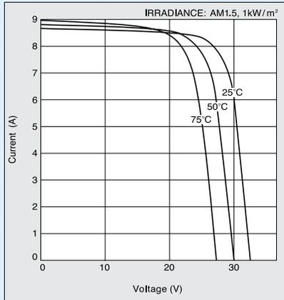
Current-Voltage characteristics of Photovoltaic Module KD215GX-LPU at various irradiance levels
