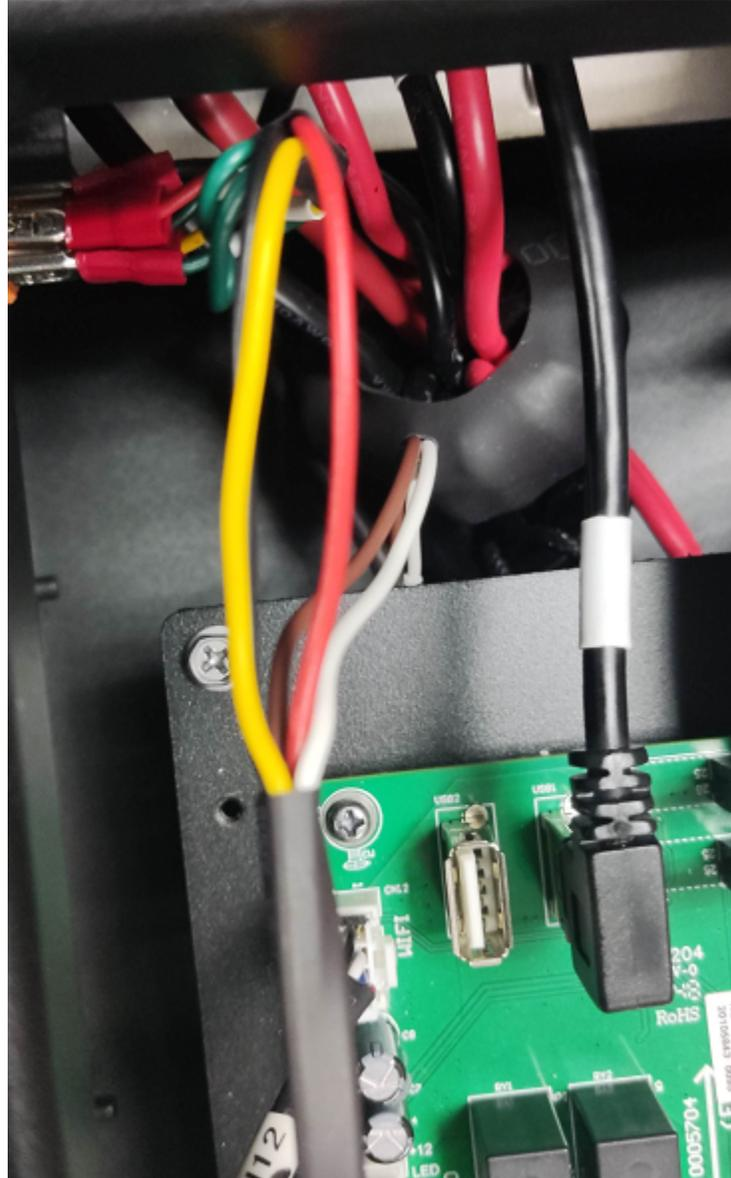
2. Step of connecting an external RSD Switch
