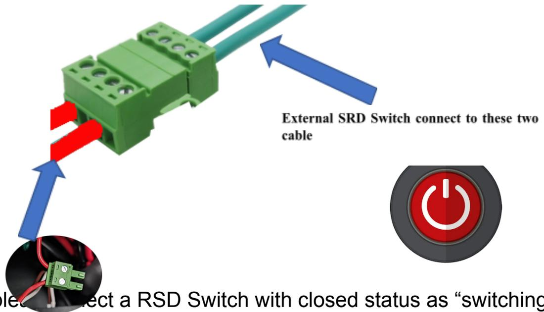
Note: please select a RSD Switch with closed status as “switching on condition”. The system will keep on normal working condition if the External RSD Switch stay in closed status, while the Rapid Shut Down will take action while the External RSD Switch is in the status of opening.
