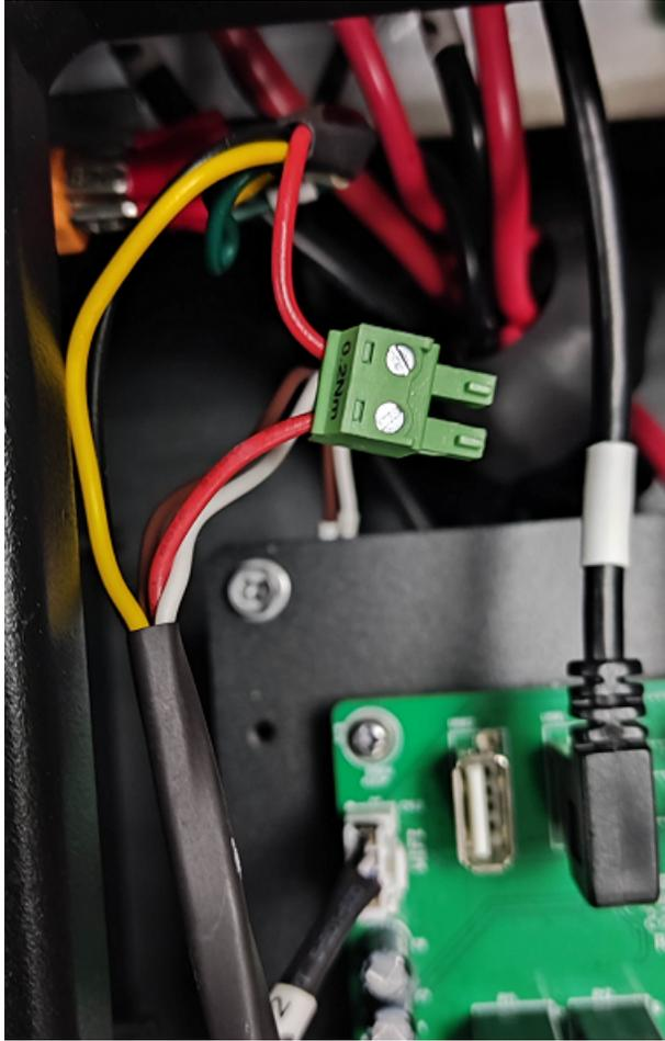
TIPS: The connectors that are used to modify the Live Line and connected an external RSD Switch include a male terminal and a female terminal, as shown in following:
