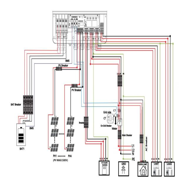
In the occasion without generator use, we recommend the user to use the generator terminal to be connected. The power of PV inverters or micro inverters can be measured by the internal sensor of the hybrid inverter.
