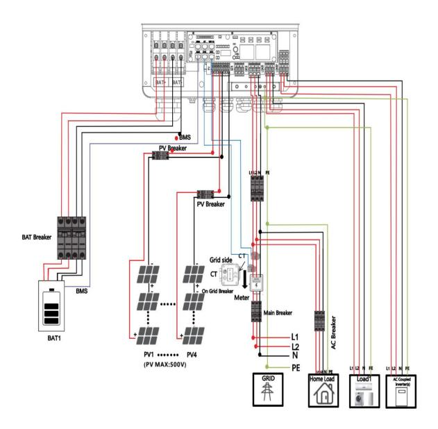
In the occasion with generator use, we recommend the user to use the load2 terminal to be connected. The hybrid inverter may not able to show the load power correctly in this case. The hybrid inverter will automatically switch off the AC Coupled inverters while the generator needs to be used.
