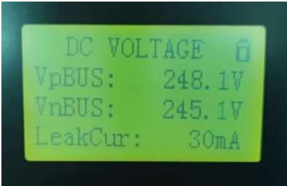
The DC BUS voltage is the DC bus voltage inside the inverter (the DC bus voltage after the PV input is tracked and transformed by the MPPT)
