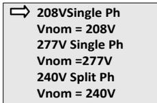
To choose a single phase 208V grid connection, move the cursor to the **208V Single Ph** line and press the [ENTER] button to open the following sub-menu:
