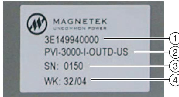
The identification plate present on the inverter includes the following data:
