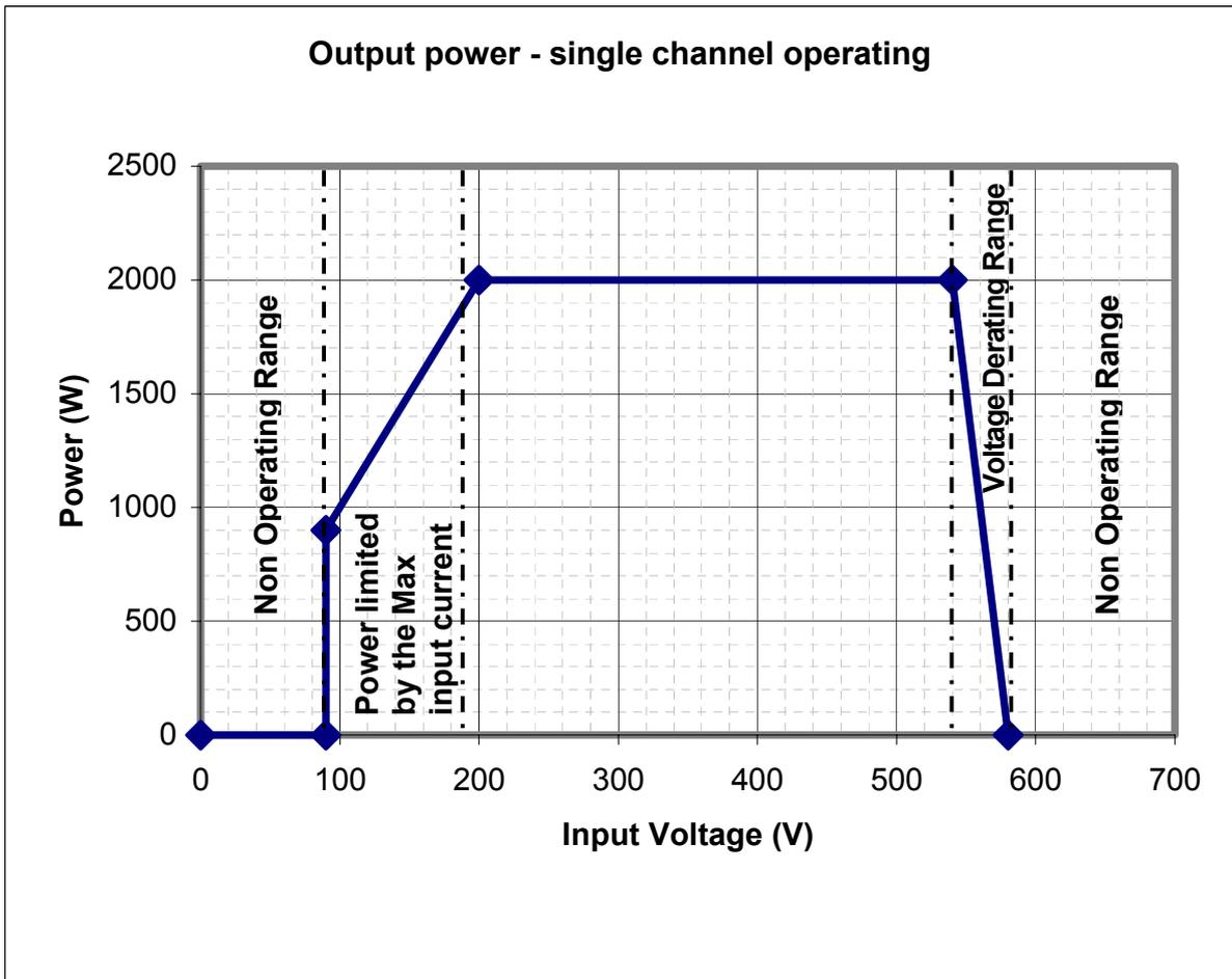
The two above cases, originating a power derating, can also occur at the same time, but the power derating will always correspond to the lowest value read.
