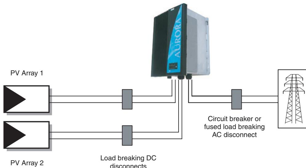
Fig.3 Simplified diagram of a photovoltaic system
