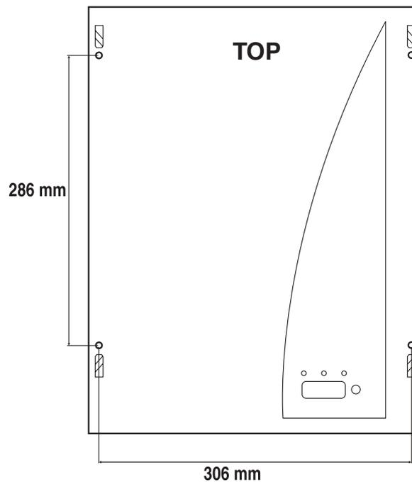
Fig.6 Wall mounting diagram
