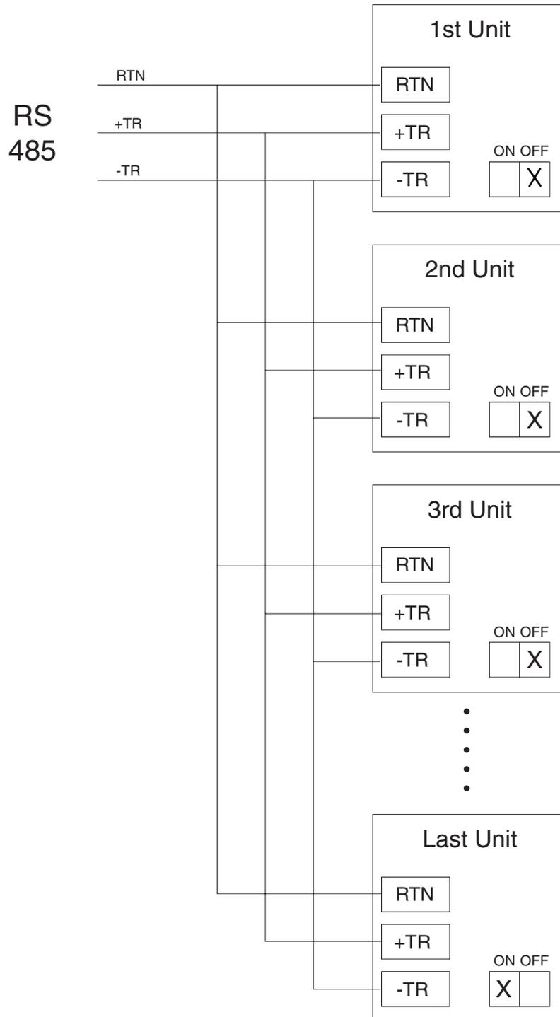
Fig.18 Multiple units connection
