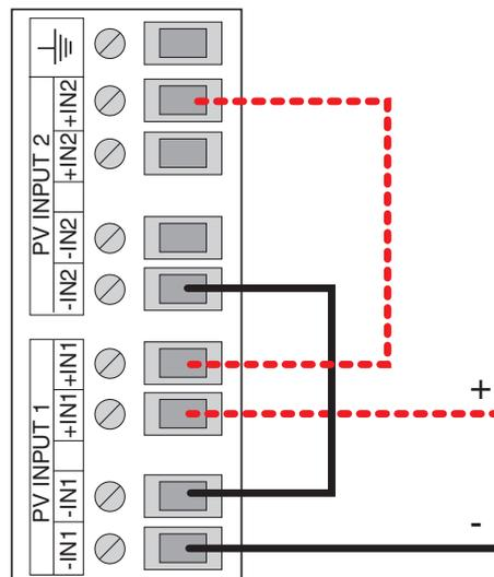
Fig.14: Paralleling the two input sections
