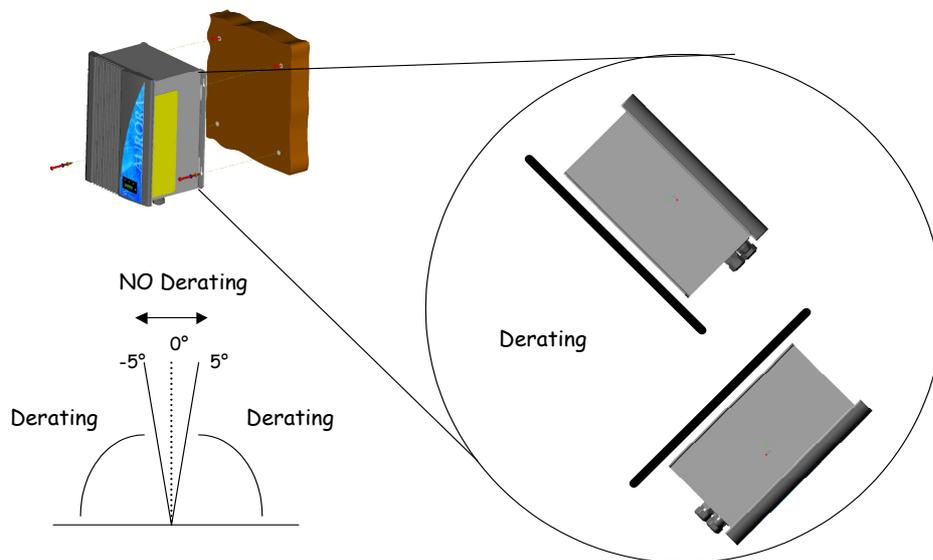
Fig.8 Inverter tilted mounting
