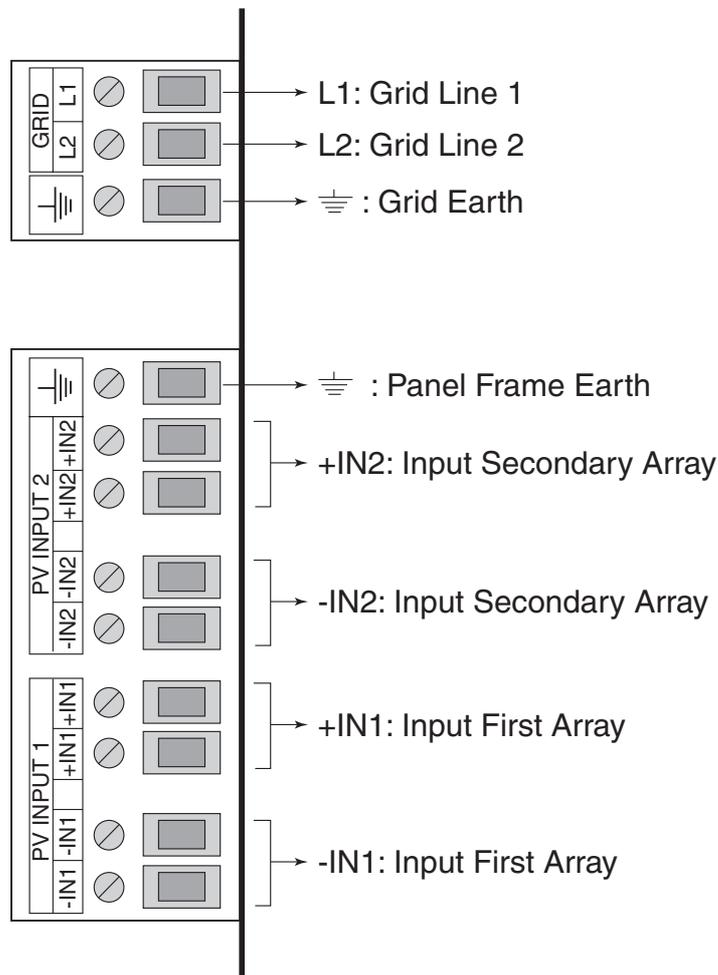
Fig 12: Screw terminal blocks
