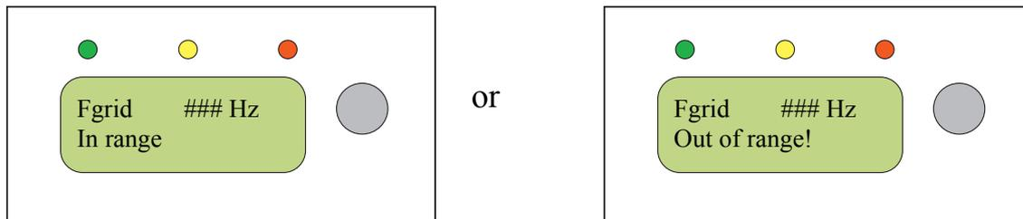
After AURORA is connected to the grid the display starts showing cyclically the following information screens, each for 5 seconds:
