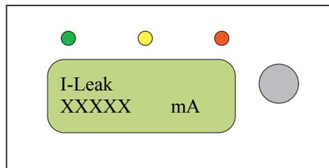
In case the inverter is not working properly the Fault or Ground Fault LEDs will turn on as described in paragraph 5.3, and the following three screens scroll on the LCD remaining on for 5 seconds. They contain important information that should be communicated to service personnel and will show cyclically on the LCD, each for 5 seconds:
