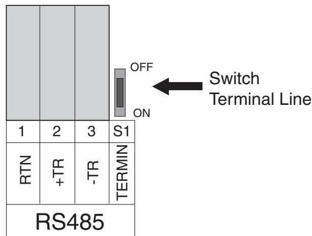
Fig.17: The RS-485 serial link terminal blocks
