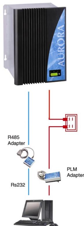
Fig.19: Data transmission to a PC
