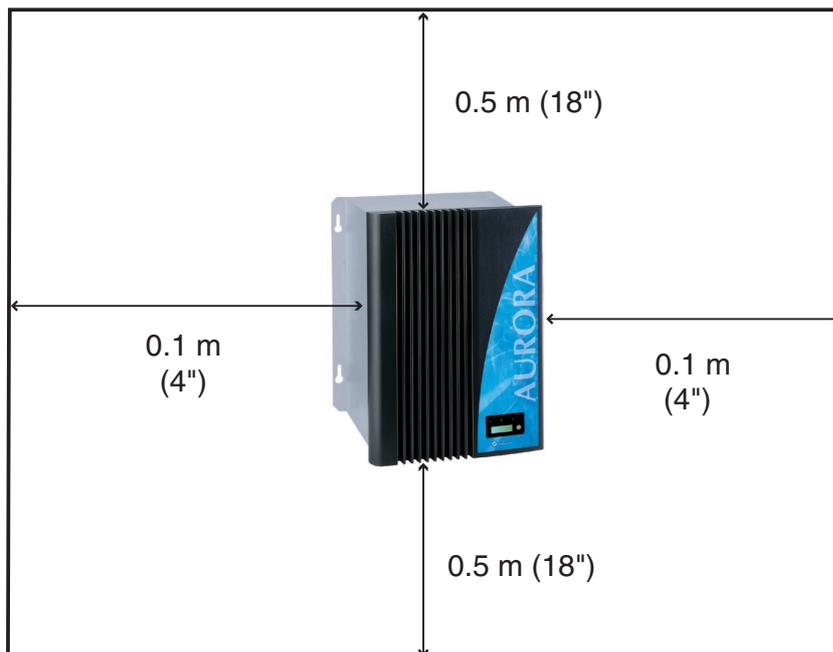
Fig.5 Minimum clearance requirements
