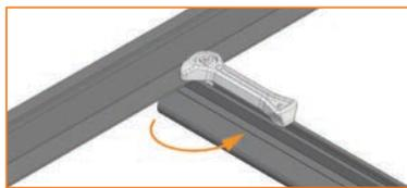
**Fig. 4b:** modules attached to supporting structure (rail, item 01) using a clamp (item 02) fixed with a bolt (item 03) and nut (item 04) – view between two modules.
