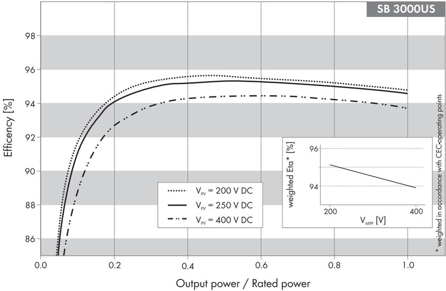
Figure 30: Efficiency curve SB 3000US/3000US-12
