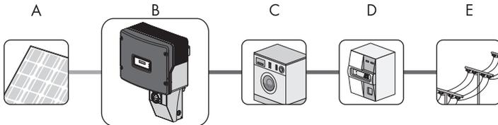
Figure 1: Principle of a PV plant with Sunny Boy
