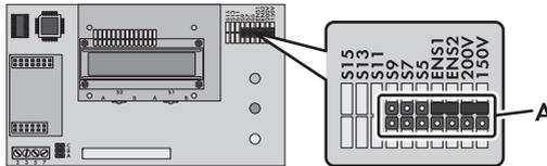
Figure 23: Pin header for setting the jumper
