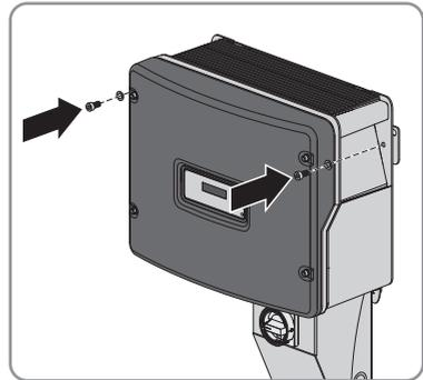
3. Close the recessed grips with the ventilation grids. Ensure that the side assignment is correct. Each ventilation grid is assigned to a side of the enclosure: Left side "links/left" and right side "rechts/right".
