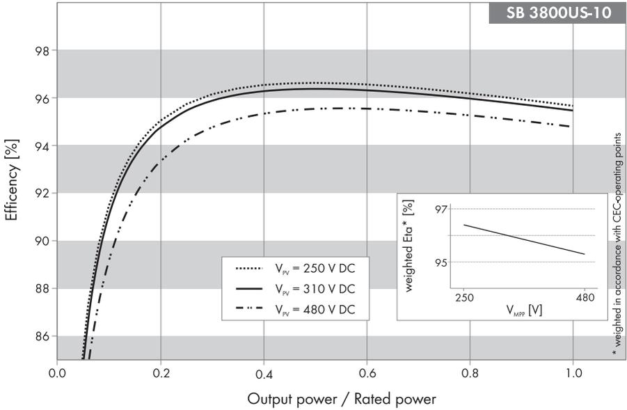
Figure 31: Efficiency curve SB 3800-US-10/3800-US-12
