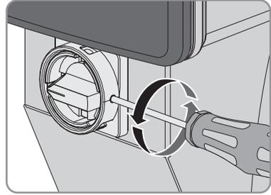
5. Remove the screw and conical spring washer of the cover on the underside of the DC Disconnect.
