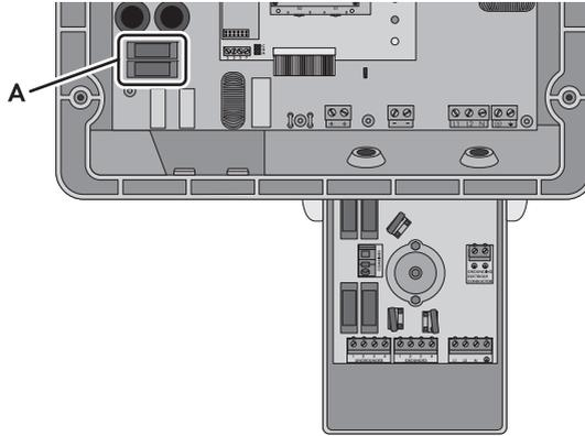
Figure 28: Position of the ground fuse
