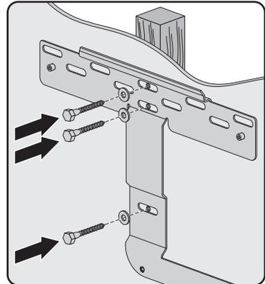
8. Tighten the screws. Ensure that no screws are loose.
