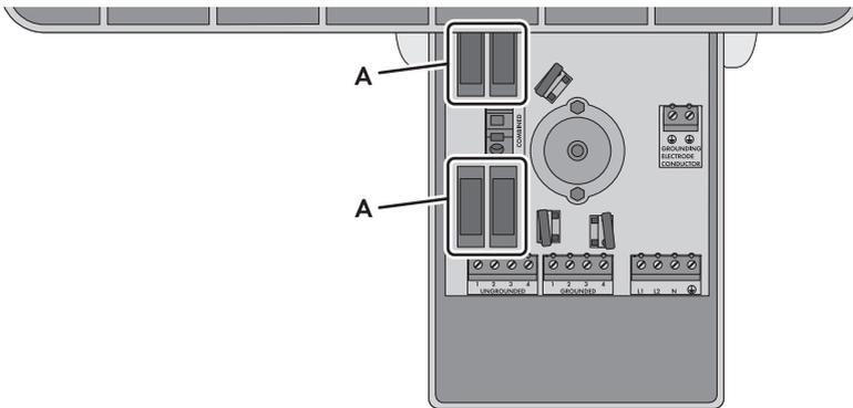
Figure 29: Position of the string fuses
