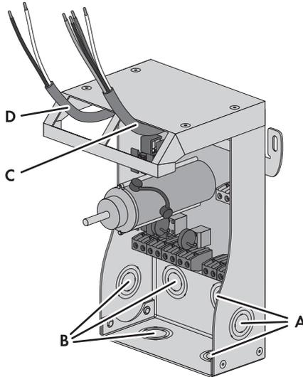
Figure 14: Connection Area of the DC Disconnect
