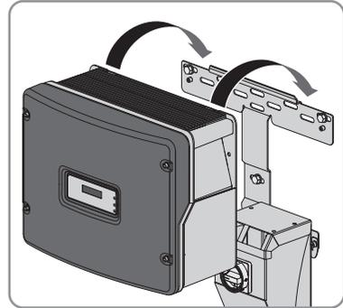
2. Screw the inverter onto the wall mounting bracket on both sides using the provided screws with conical spring washers (torque: 44 in-lb. (5 Nm)).
