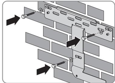
9. Tighten the screws. Ensure that no screws are loose.
