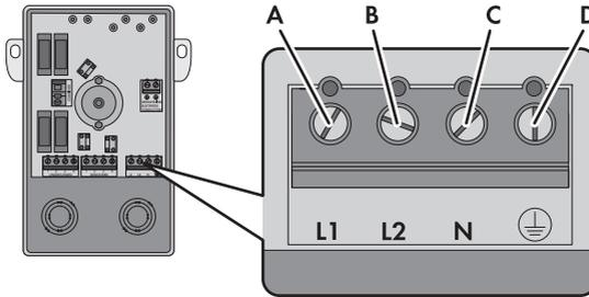
Figure 15: AC connecting terminal plate for connecting the power distribution grid
