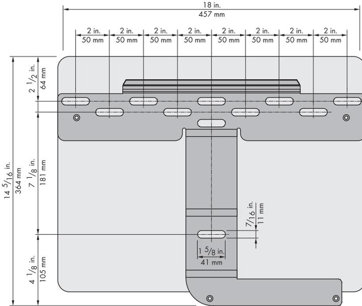
Figure 8: Dimensions of the wall mounting bracket
