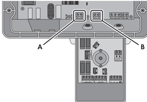
Figure 20: DC+ and DC – connecting terminal plates for connecting the DC cable of the DC Disconnect
