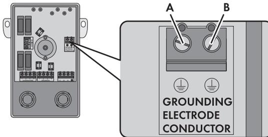
Figure 17: Connecting terminal plate for connecting the protective conductor
