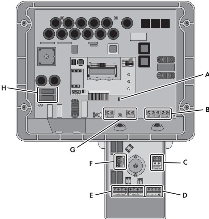
Figure 12: Components and connection areas in the interior of the inverter and the DC Disconnect
