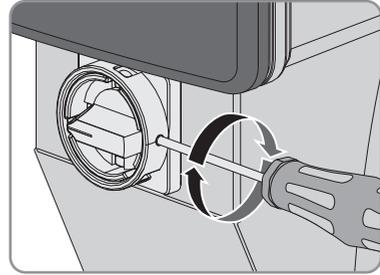
6. Attach the conical spring washer on the screw of the DC Disconnect. Here, the grooved side of the conical spring washer must point to the screw head.
