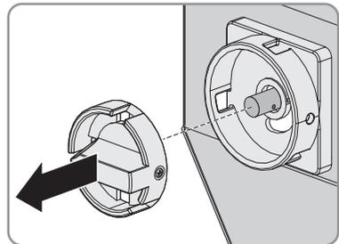
7. Remove the cover of the DC Disconnect.
