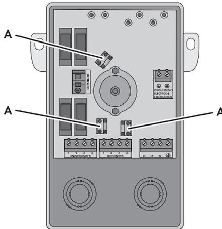
Figure 11: Position of terminals for the DC varistors
