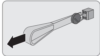
6. Ensure that all DC varistors in the terminals are securely in place.
