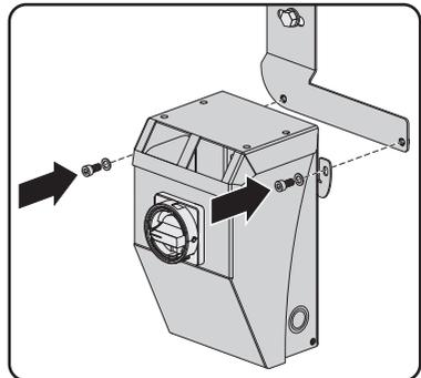
2. Tighten the screws (torque: 44 in-lb. (5 Nm)).
