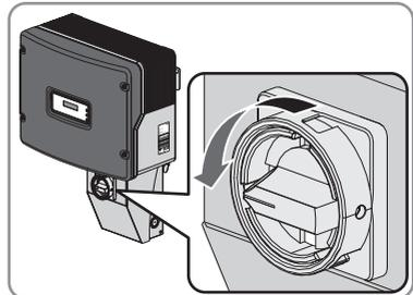
3. If additional DC switch-disconnectors are available, switch off the DC switch-disconnectors and secure against re-connection.
