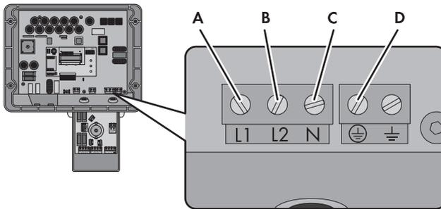
Figure 16: AC connecting terminal plate for connecting the AC cable of the DC Disconnect
