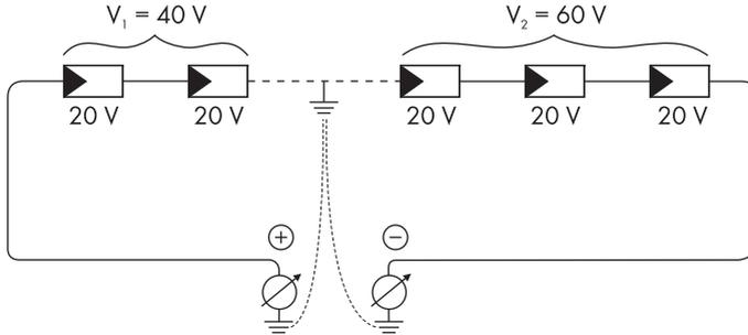
Figure 27: ground-fault in the PV array
