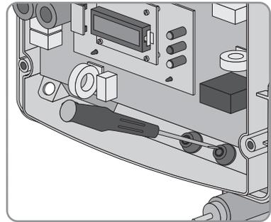
3. Insert the DC cable of the DC Disconnect into the inverter through the rubber grommet.
