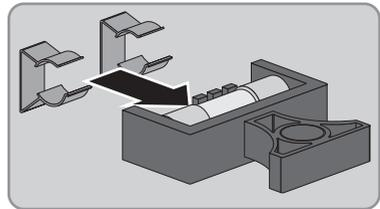
3. Remove defective ground fuse from the fuse extractor and insert a new ground fuse into the fuse extractor. Ensure that the ground fuse is functional and is the correct size.
