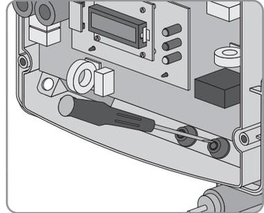
3. Insert the AC cable of the DC disconnect into the inverter through the rubber grommet.
