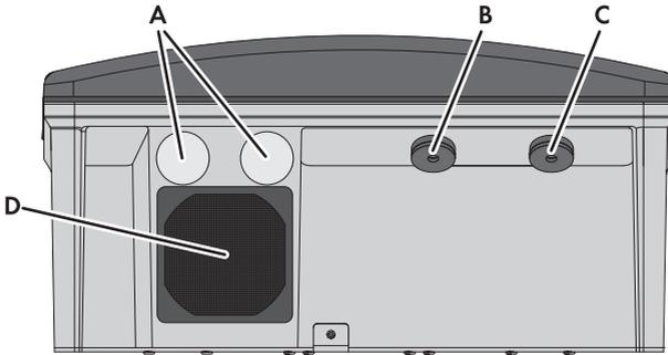
Figure 13: Terminals on the underside of the inverter
