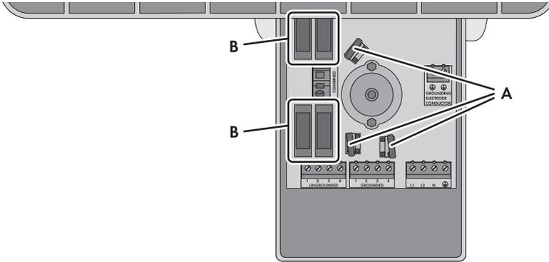
Figure 26: Position of the DC varistors and string fuses
