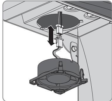
6. Insert the fan into the inverter until the fan audibly snaps into place.
