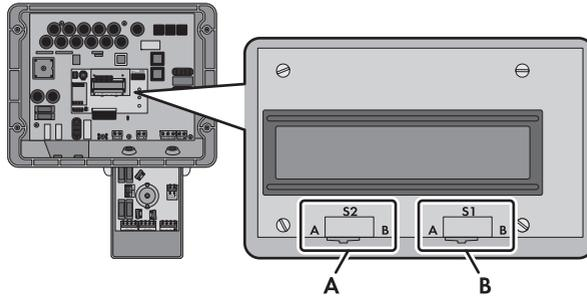
Figure 24: Switch for setting the language on the bottom edge of the display
