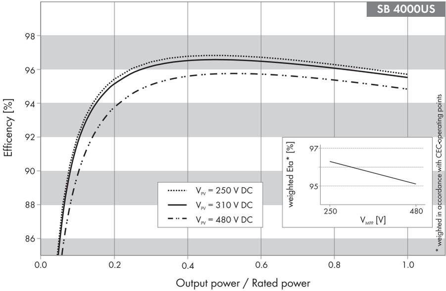
Figure 32: Efficiency curve SB 4000US/4000US-12
