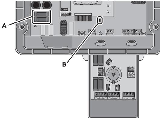
Figure 18: Position of fuse holder for fuse extractor with ground fuse and pin header for jumper
