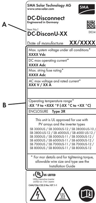
Figure 5: Layout of the DC Disconnect type label
