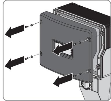
5. The enclosure lid, screws, and conical spring washers are to be stored safely.
