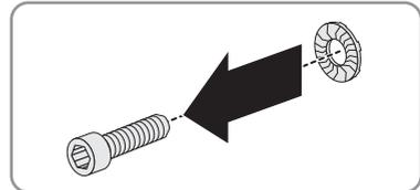
7. Insert the screw and conical spring washer into the underside of the DC Disconnect and tighten the screw (torque: 44 in-lb. (5 Nm)). Ensure that the toothing of the conical spring washer points towards the cover.
