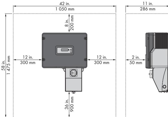
Figure 9: Recommended clearances for mounting the inverter
