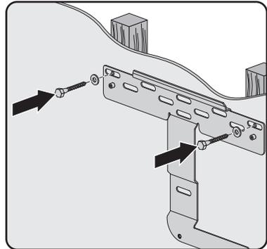
8. Tighten the screws. Ensure that no screws are loose.
