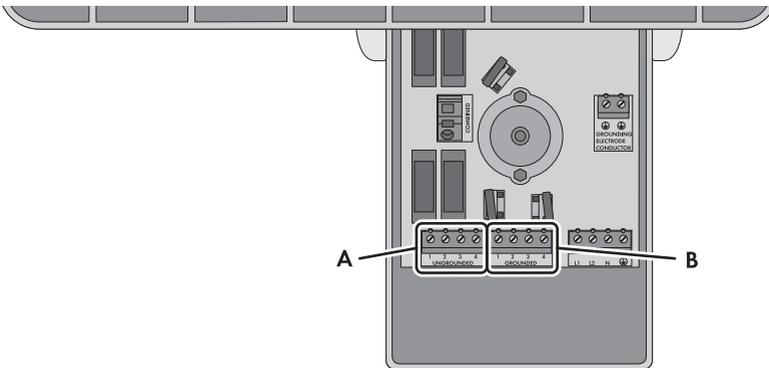
Figure 19: DC connecting terminal plates for connecting the PV array
