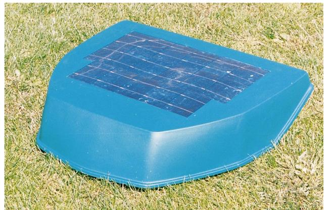
*An ultralight Solarex custom laminate powers a robotic lawnmower.*
