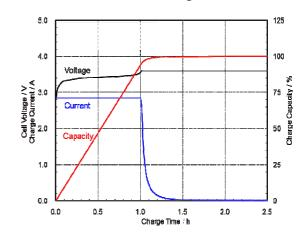
\*Charge at 1ltA rate under ambient temperature of 23 deg. C
