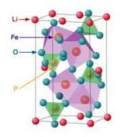
\*With its covalently bonding crystal structure, the cathode material does not release oxygen easily even under high ambient temperature and prevents thermal runaway
