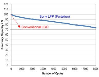
\*1ItA charge / discharge full cycles (100% DOD) at 23 deg. C
