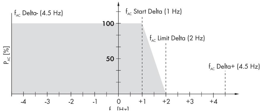
Figure 1: Operating principle of FSPC
