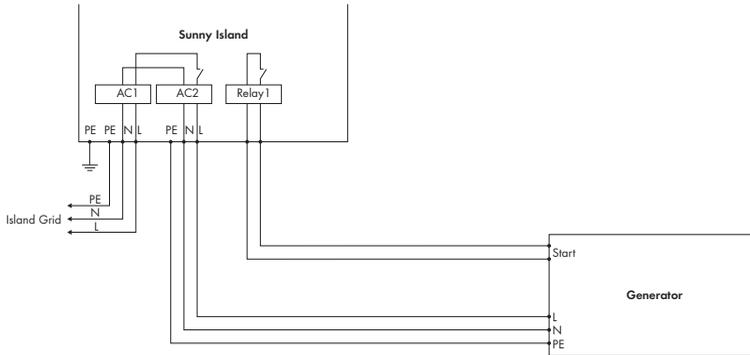
If you directly start the generator manually in this operating mode, the Sunny Island 5048U detects the running generator and connects it once the warm up time has expired. If you stop the generator externally, this is detected and the generator is disconnected and the stand-alone grid continues to be powered.
