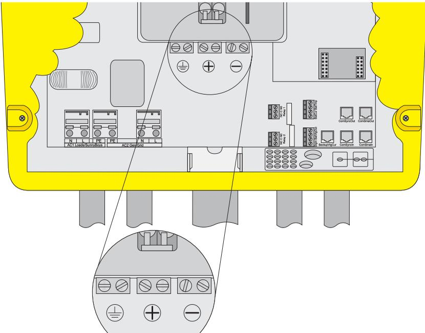
1. Install a 1 1/2-inch conduit fitting in the Sunny Island 5048U wiring knockout (the knockout on the middle). Fasten the conduit fitting on the inside of the Sunny Island 5048U with the appropriate locknut.
