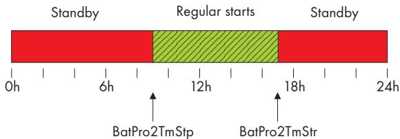
**Level 3:** The third level ensures that the battery is protected from deep discharge and thus protected against damage. In this case, the inverter is switched off completely. To start the inverter, please see section 9.5 "Reactivating the Device Following Automatic Shutdown" (Page 68).
