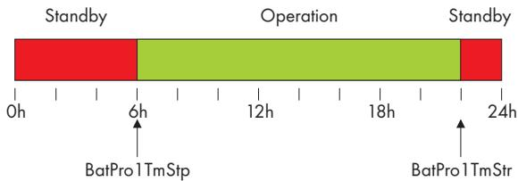
**Level 2:** The second level of the battery preservation mode ensures that the inverter regularly starts every two hours but only during the window of time in which an energy supply is expected and attempts to charge the battery from the AC side. For photovoltaic systems, this occurs during the day. In this case, you define the start time using the "223.03 BatPro2TmStr" parameter and the stop time using the "223.04 BatPro2TmStp" parameter.
