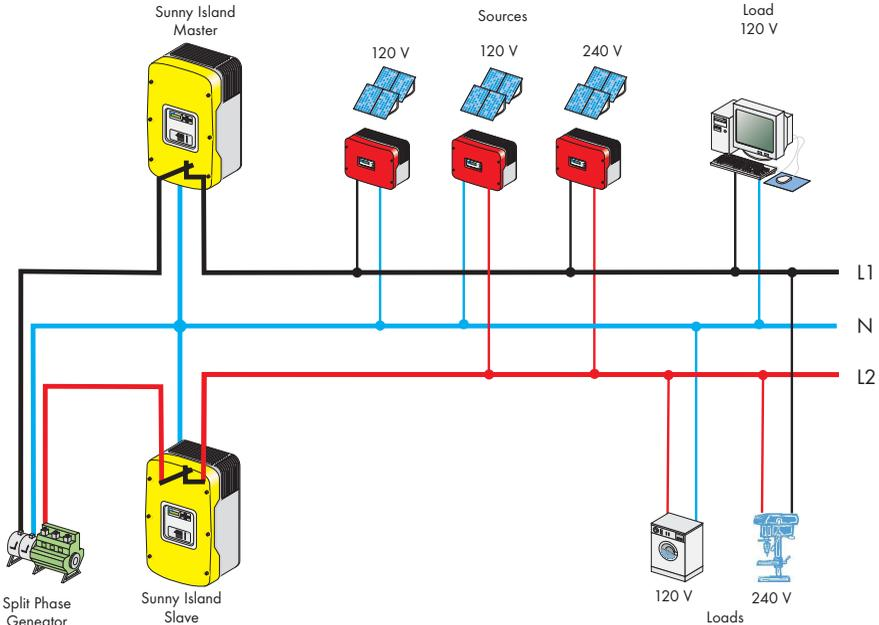
Generally speaking the relays of the slave unit will only close when the master relay also closes.
