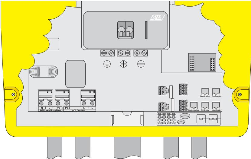
Use the provided terminal blocks to fasten the cables inside the Sunny Island 5048U housing in a manner conforming to the appropriate standards. The metric-thread cable screw connections guarantee a dust-free and waterproof installation of the cables in the housing and also provide strain relief for the cable connection. Close all unused openings in the housing using the appropriate dummy plugs (the dummy plugs are already installed on AC2 and DC-Ground upon delivery).
