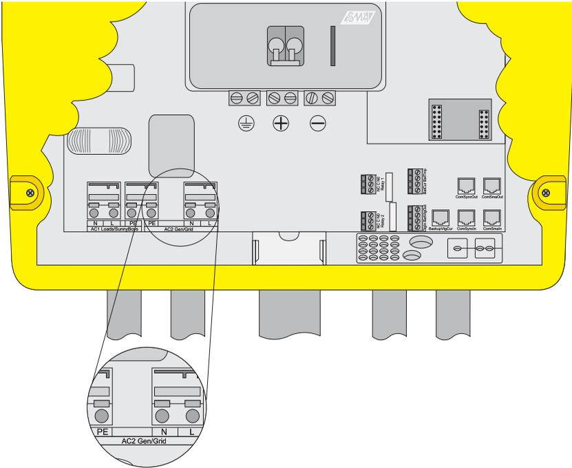
1. Install a 3/4-inch conduit fitting in the Sunny Island 5048U wiring knockout (the knockout on the left side). Fasten the conduit fitting on the inside of the Sunny Island 5048U with the appropriate locknut.
