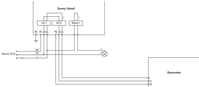
The generator is also always switched off manually. The Sunny Island 5048U then automatically switches into the operating mode without the generator.
