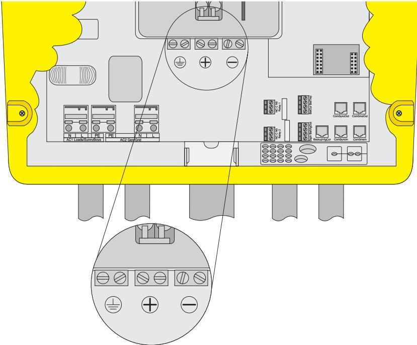
1. Install a 1 1/2-inch conduit fitting in the Sunny Island 5048U wiring knockout (the knockout on the middle) or at the battery enclosure. Fasten the conduit fitting on the inside of the Sunny Island 5048U with the appropriate locknut.
