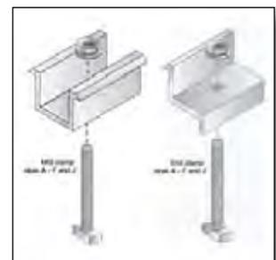
SolarMount Top Mounting Clamps
