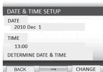
4 After entering the DATE and TIME, select "DETERMINE DATE AND TIME" using [→] and press [ENTER].
