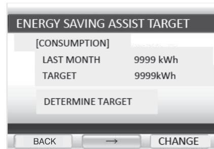
4 Select “DETERMINE TARGET” using [→] and press [ENTER].
