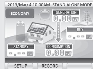
When the storage battery charge is low, power is supplied entirely from the solar panels.
