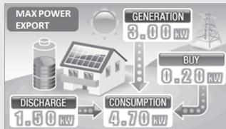
The storage batteries are discharged to supplement power shortages (when power is purchased from the power company) during the daytime hours up until the nighttime hours begin. \*1, 2, 3, 4, 7
