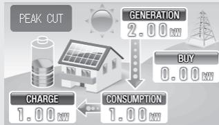
If the amount of sunlight increases, surplus solar power is used to charge the storage batteries.
