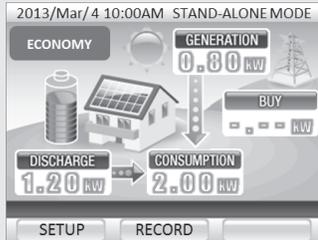
The storage batteries are discharged to supplement power shortages when there is an insufficient amount of sunlight.
