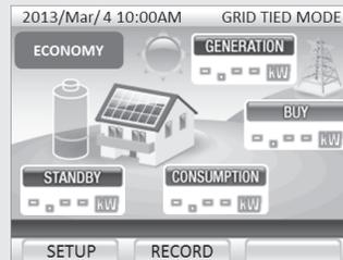
If power is restored on the commercial power grid while the Remote Controller is out, the Remote Controller indicates "GRID TIED MODE" as the operating status.
