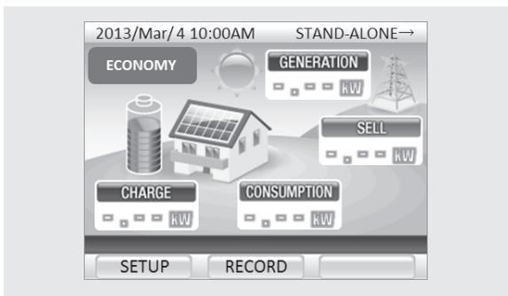
**3** After about 10 seconds, the Remote Controller automatically changes the operating status message to “STAND-ALONE MODE”.
