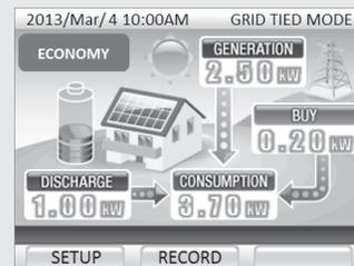
Once the storage batteries are fully charged, grid-tied operation starts from the set operating mode.
