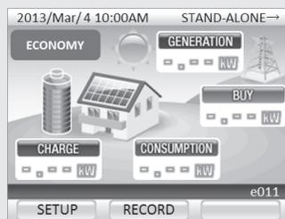
If power consumption exceeds power output, stand-alone operation temporarily stops. \*2
