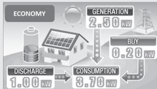
The storage batteries are discharged to supplement power shortages (when power is purchased from the power company). \*2, 3, 4, 7
