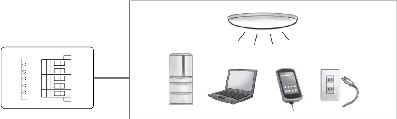
Circuitry has been designed to enable lighting fixtures, communication equipment and other electric appliances to be used in the event of a power outage without having to unplug and plug them back in again.
