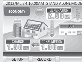
If the amount of sunlight increases, surplus solar power is used to charge the storage batteries. \*1
