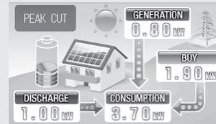
The storage batteries are discharged to supplement power shortages (Discharges in order to cut peak). \*2, 3, 4, 7
