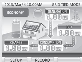
Once power is restored on the commercial power grid and the inverter engages grid-tied operation, the amount of power used during the power outage is recharged to the storage battery.
