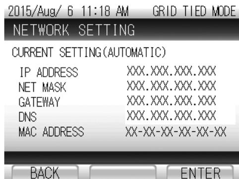
This completes the procedure to perform automatic configuration of network settings. Follow the procedure described in “4. Setting REMOTE MONITOR, Performing the communication test” (Page 46) to test the connection.
