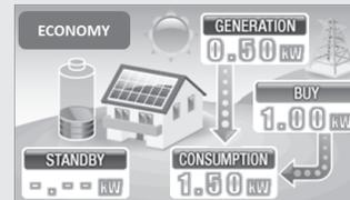
If there is an insufficient amount of sunlight and the storage batteries are low, charging/discharging is stopped. \*2, 4
