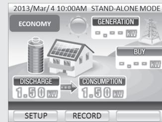
If there is an insufficient amount of sunlight, power is supplied entirely from the storage batteries. \*3
