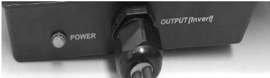
**5. Attach the OUTPUT [Invert] connectors to the cables from the inverter.**
