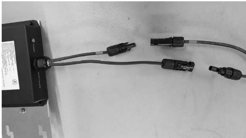
**ATTENTION** A home run length of greater than 150 feet for any individual home run will negate the safety functionality of the device. A home run refers to the cable between the PV array and the inverter.
