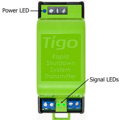
Verify that the transmitter is working correctly:
