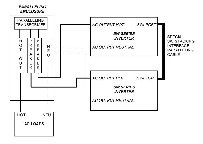
Each inverter should have its own DC overcurrent protection device (breaker or fuse). The DC negative terminals of the inverter should be connected close to the inverters (within 36" / 1 meter of cable). This is important for proper operation of the intercommunication system of the inverters. If longer battery cables are required, add another heavy cable between the two inverters DC negative terminals as short as possible.
