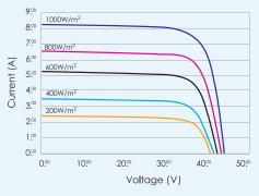
Average efficiency reduction of 4.5% at 200W/m $^{2}$  according to EN 60904-1.
