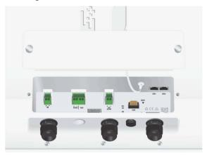
2. Remove the grommet from the SolarBeam.
