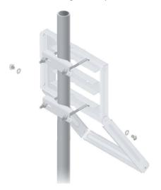
4. Insert the Panel into the Mounting Bracket and Strut.
