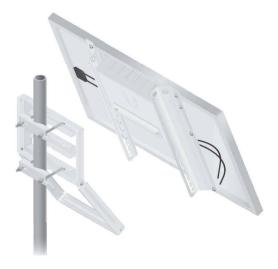
5. Attach the *Panel* to the *Mounting Bracket* and *Strut* using four *Flat Washers* and *Bracket Screws*. Hand-tighten only.
