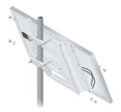
6. Adjust the angle of the *Panel* based on your latitude (refer to the *Installation Guidelines* section on page 5). Then tighten the six *Bracket Screws* to 17 N·m.
