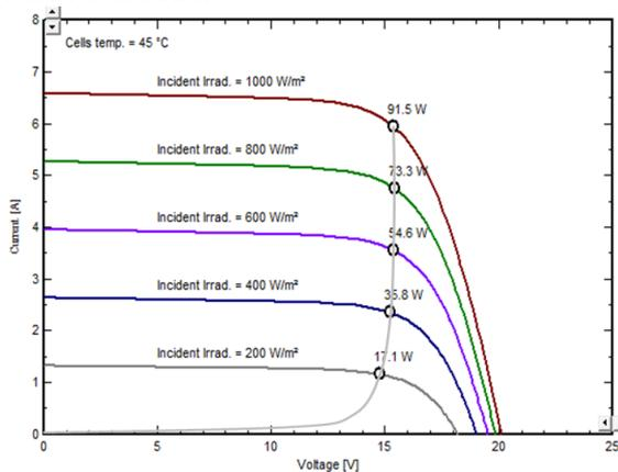
Figure 16: Dependence of  $M_p$  and  $V_{mp}$  on irradiance
