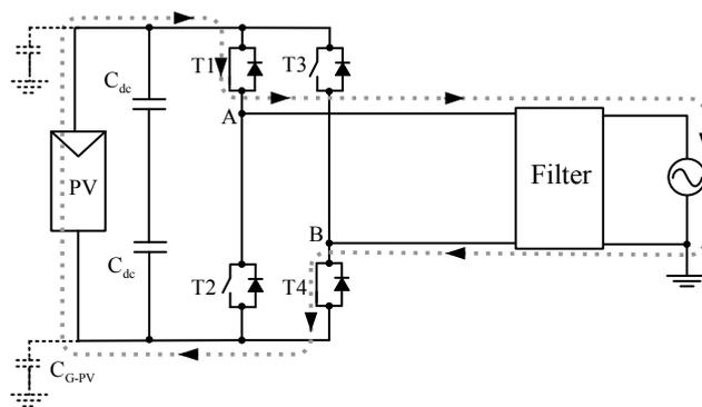
Fig. 3.4: T1-T4 turned-ON, for  $+V_{DC}$  output voltage.
