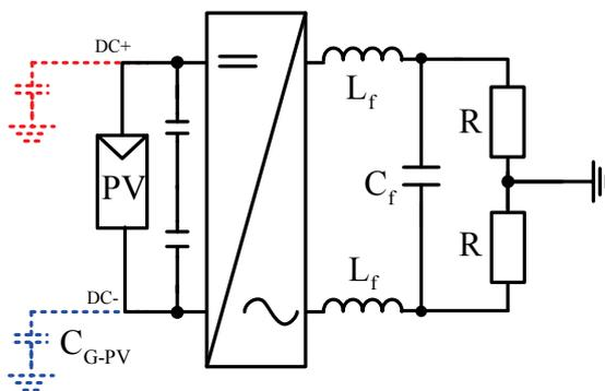
Fig. 5.1: Test setup used for common-mode voltage measurement.
