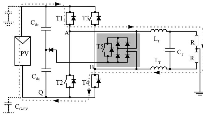
Fig. 5.10. HB-ZVR topology, active vector applied to load, using T1-T4, during positive half-wave.
