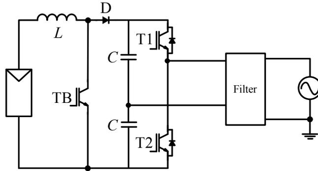
Fig. 2.9: Half-bridge topology with voltage boost stage [38].
