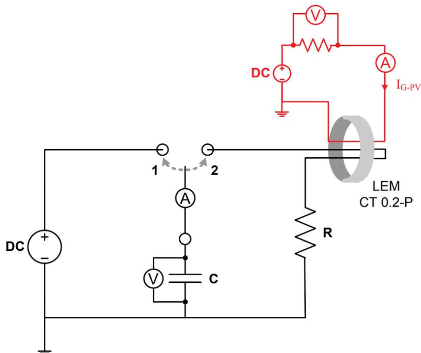
Fig. A.5 Laboratory test-setup for discharge test for the LEM CT 0.2-P
