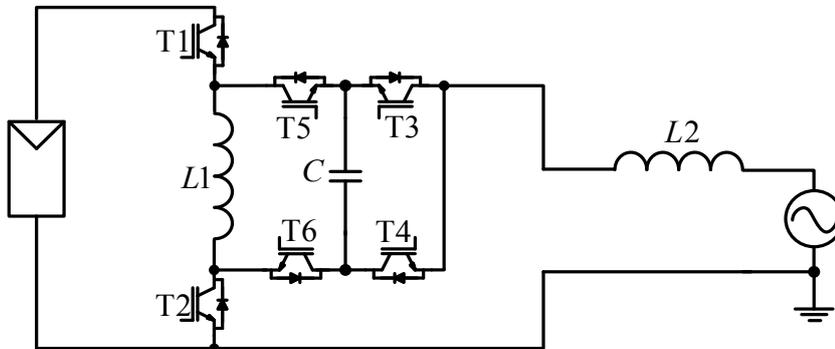
Fig. 2.16: Transformerless PV inverter topology patented by Schekulin [47].
