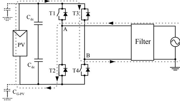
Fig. 3.5: T2-T3 turned-ON, for  $-V_{DC}$  output voltage.
