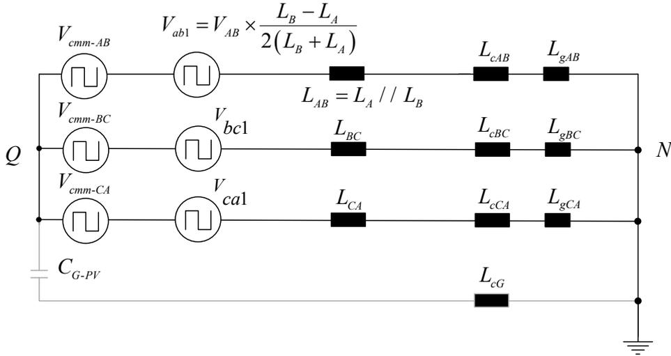
Fig.4.4. Simple model showing the common mode voltage for the three-phase system.
