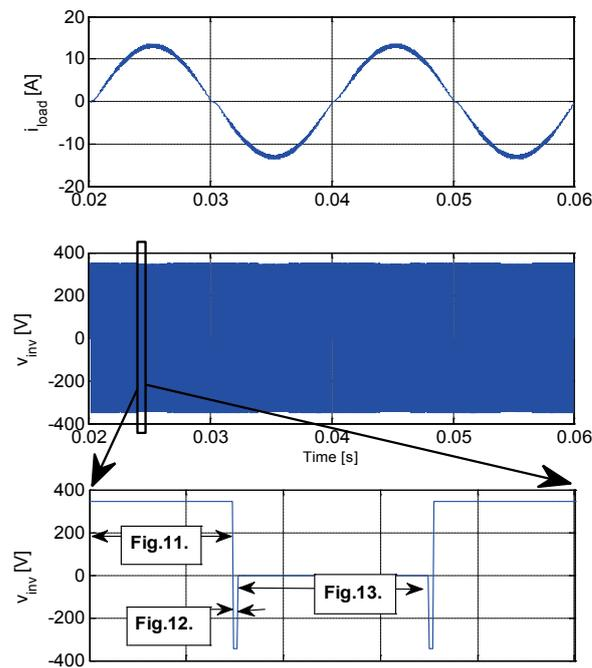
Fig. 5.13. HB-ZVR load current and inverter output voltage.
