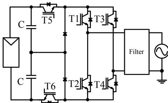
Fig. 2.20: Transformerless topology by Gonzales et al. [53].
