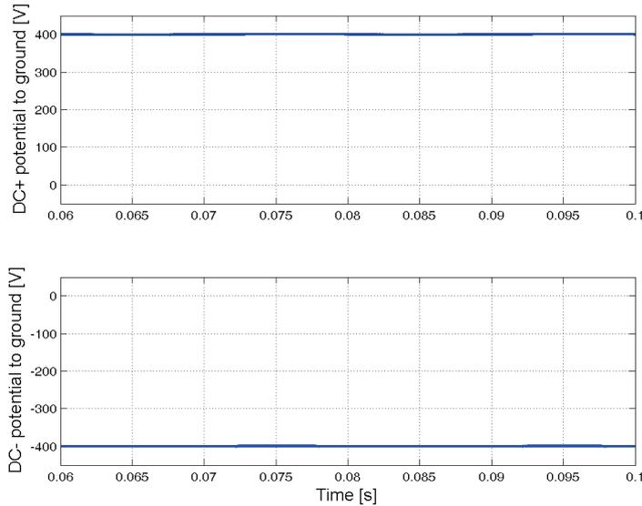
Fig. 3.21: Voltage to ground for both terminals of the PV array for the NPC topology.
