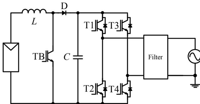
Fig. 2.8: Transformerless PV inverter with voltage boost stage [37].
