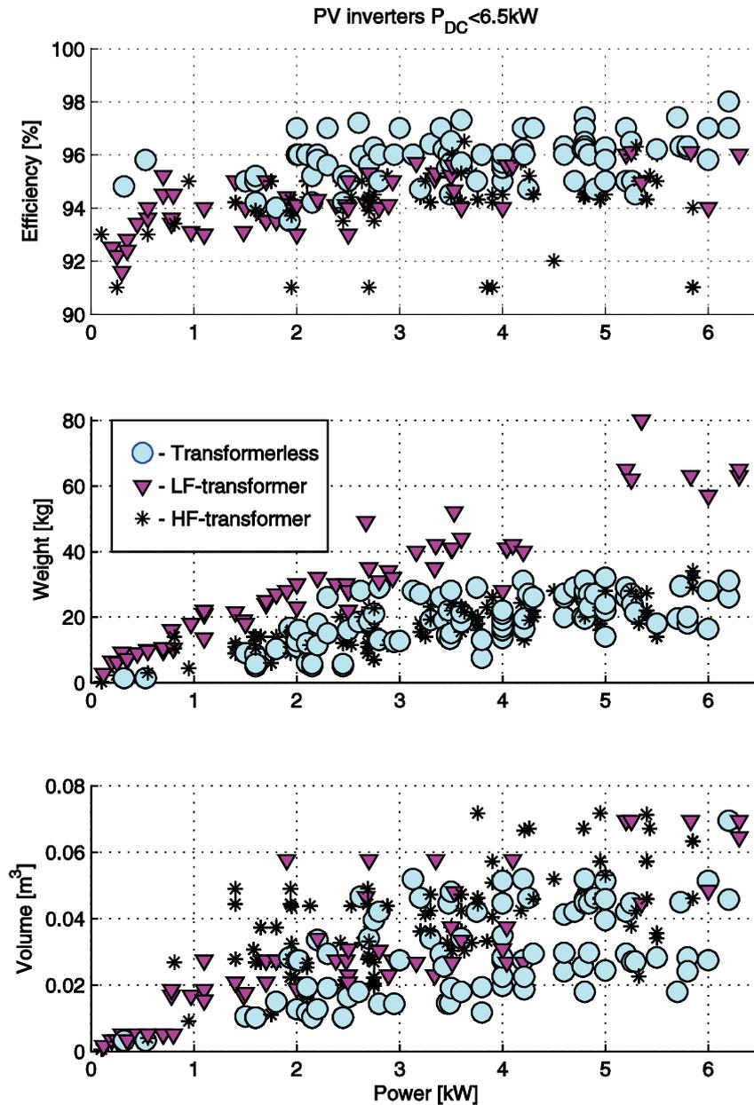
Fig. 2.5: PV inverter comparison, based on PHOTON database.
