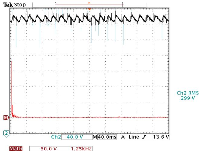
Fig. 4.11: DC to ground voltage (Channel 2) [40V/div] and FFT of the same voltage (Channel M) having 1.25 kHz per division on the FFT.
