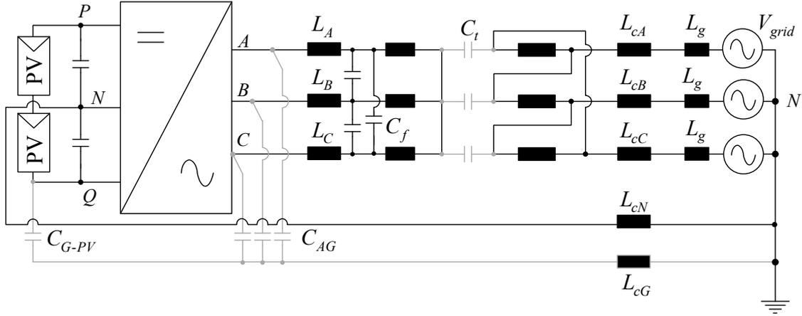
Fig.4.2. Three-phase grid-connected PV system showing the parasitic capacitance of the PV array, the parasitic capacitance of the converter, the cable inductance of the phases, and the stray capacitance of the transformer in a system with galvanic isolation.
