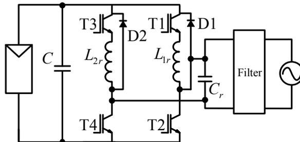
Fig. 2.13: Four-switch resonant buck-boost inverter by Wang [45].
