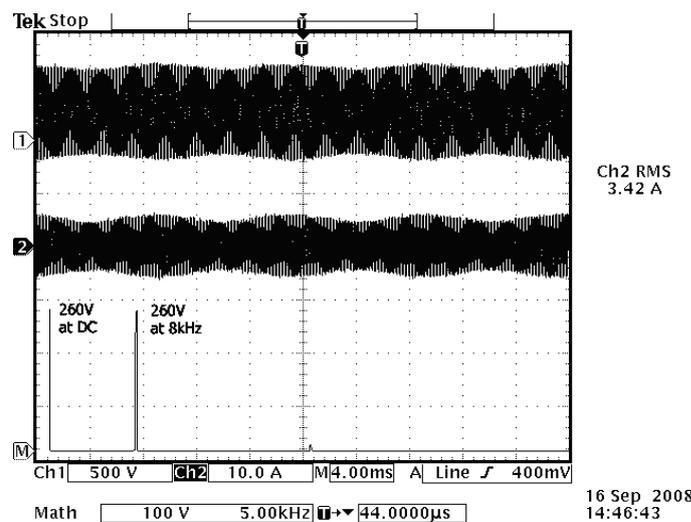
Fig. 5.16. Experimental results for H-Bridge topology with unipolar PWM, Channel 1 shows the voltage to ground of the DC+ terminal, Channel 2 shows the ground leakage current and Channel M shows the voltage to ground of the DC+ terminal.
