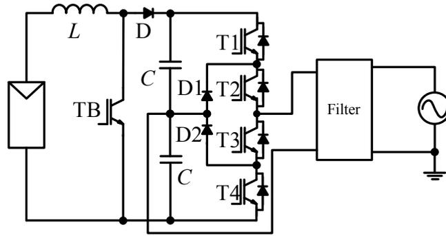
Fig. 2.17: Neutral point diode clamped inverter [37], [49] and [50].
