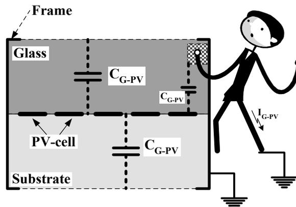
Fig. 2.21: Parasitic capacitance in PV panels [2].
