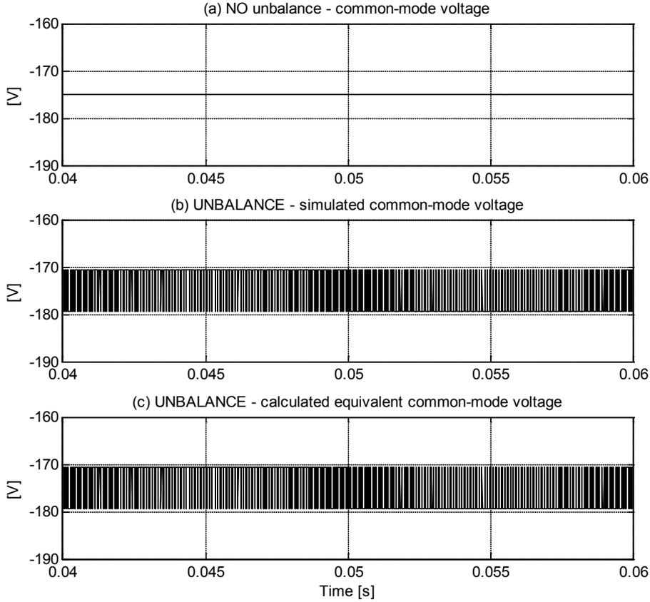
Fig. 4.13: Total common-mode voltage H-Bridge topology with bipolar PWM, (a) common-mode voltage in case of NO unbalance; (b) common-mode voltage in case of unbalance (simulation) and (c) common-mode voltage in case of unbalance (calculated) having  $L_N=0.95 \cdot L_A$  in the grid neutral.
