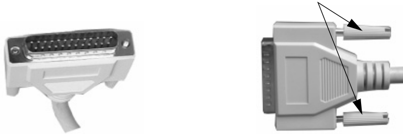
Figure 2-8 The 25-pin D-connector on the ISC-S Cable
